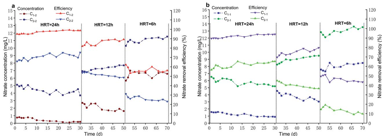
Fig. 2 Nitrate concentration and removal efficiency in column experiments. (a) Comparison between C<sub>1-2</sub> and C<sub>2-2</sub>; (b) comparison between C<sub>1-1</sub> and C<sub>2-1</sub>. (C<sub>1-1</sub>: soaked iron scraps system, C<sub>1-2</sub>: soaked both iron scraps and biochar system, C<sub>2-1</sub>: not soaked iron scraps system, C<sub>2-2</sub>: not soaked both iron scraps and biochar system).
