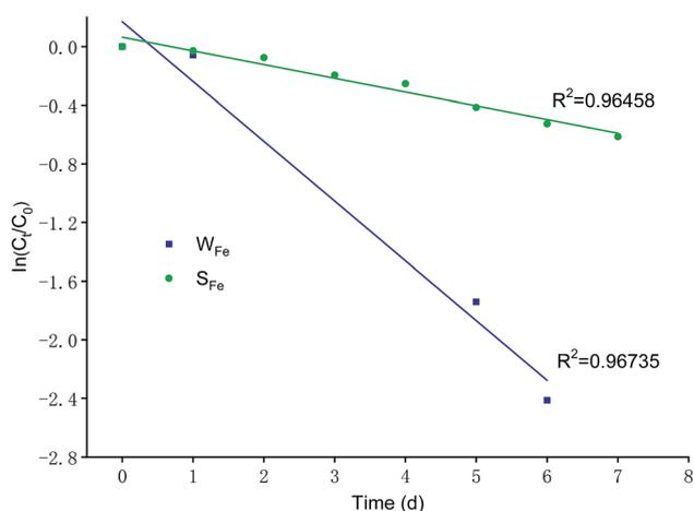
Fig. 5 Effect of microbes on nitrate removal in batch experiments. ( $C_0$ ,  $C_t$ : the initial and instant nitrate concentration,  $W_{Fe}$ : iron scraps-added wastewater system,  $S_{Fe}$ : iron scraps-added synthetic water system).
