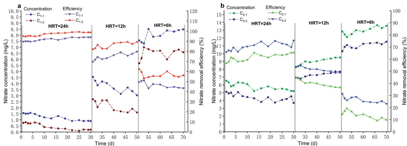
**Fig. 3** Nitrate concentration and removal efficiency in column experiments. (a) Comparison between  $C_{1-1}$  and  $C_{1-2}$ ; (b) comparison between  $C_{2-1}$  and  $C_{2-2}$ . ( $C_{1-1}$ : soaked iron scraps system,  $C_{1-2}$ : soaked both iron scraps and biochar system,  $C_{2-1}$ : not soaked iron scraps system,  $C_{2-2}$ : not soaked both iron scraps and biochar system).
