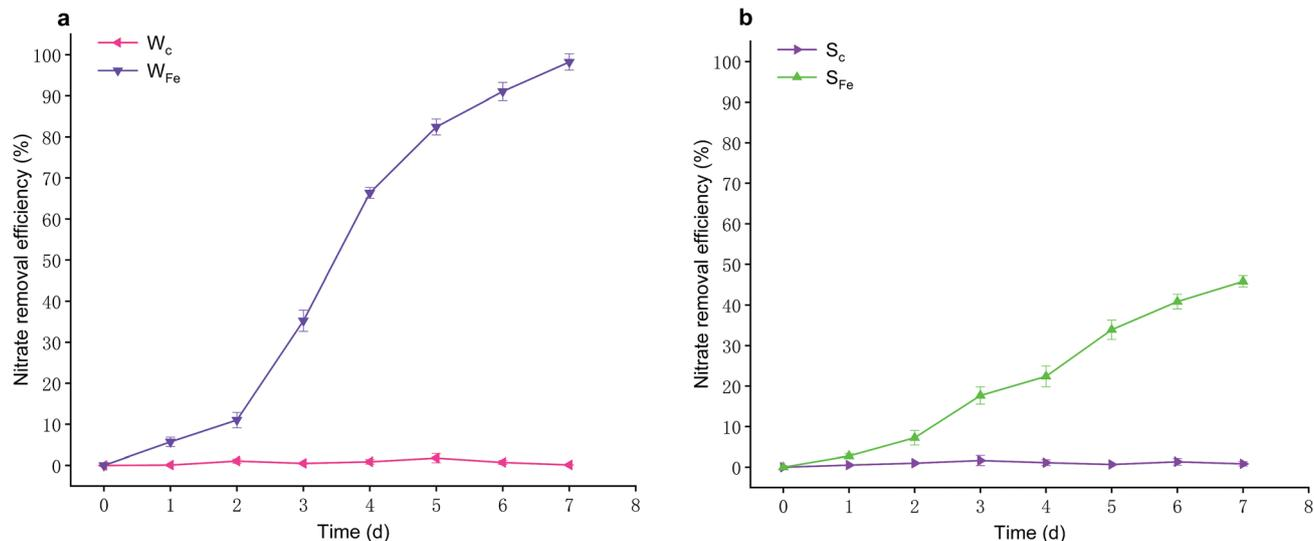
Fig. 4 Nitrate removal efficiency in batch experiments. (a) Comparison between  $W_C$  and  $W_{Fe}$ ; (b) comparison between  $S_C$  and  $S_{Fe}$ . ( $W_C$ : wastewater system,  $W_{Fe}$ : iron scraps-added wastewater system,  $S_C$ : synthetic water system,  $S_{Fe}$ : iron scraps-added synthetic water system).
