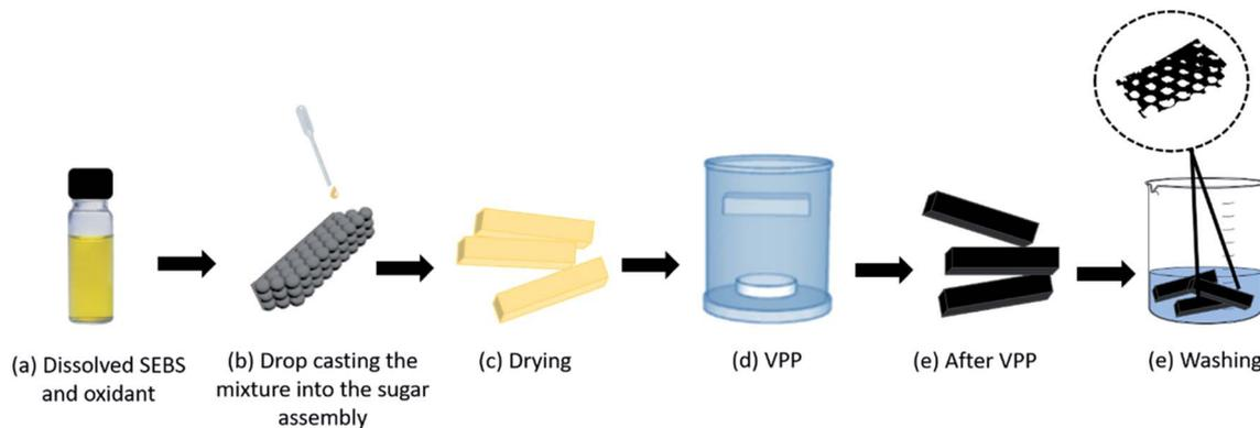
**Scheme 1** Schematic representation of the vapor-phase polymerization (VPP) of polypyrrole (PPy)-styrene-ethylene-butylene-styrene (SEBS) onto a sugar-coated silicon mold assembly in order to form a hybrid scaffold material.
