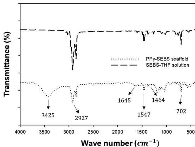
Fig. 6 FTIR spectra of the PPy-SEBS scaffold and SEBS-THF solution showing the uniform VPP deposition of PPy on the SEBS matrix.
