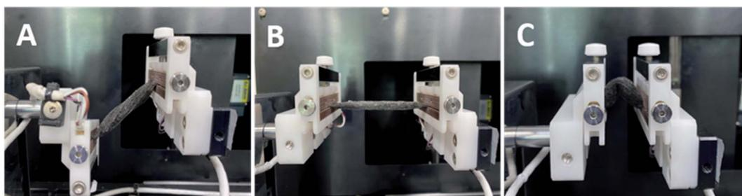
Fig. 2 Photographs during the (A) twisting, (B) stretching, and (C) bending of the PPy-SEBS hybrid scaffold.
