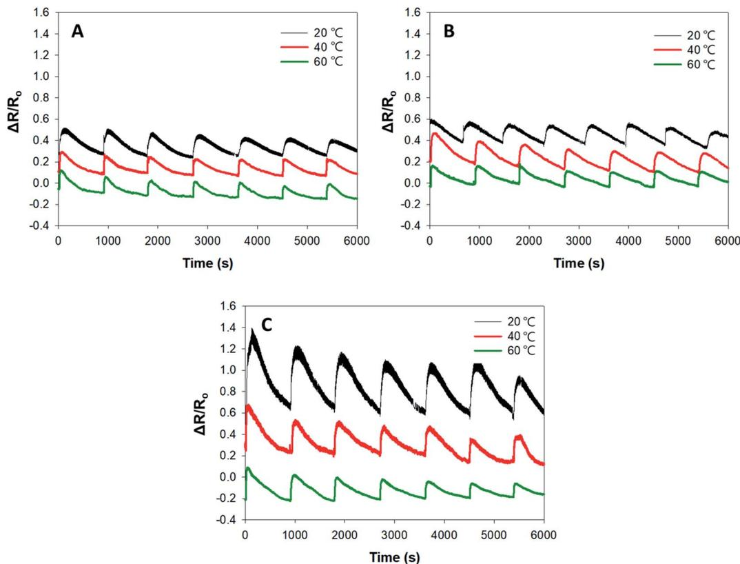
Fig. 7 Response of the (A) small-, (B) medium-, and (C) large-pore-sized PPY-SEBS hybrid scaffold to NH<sub>3</sub> gas at different operating temperatures.
