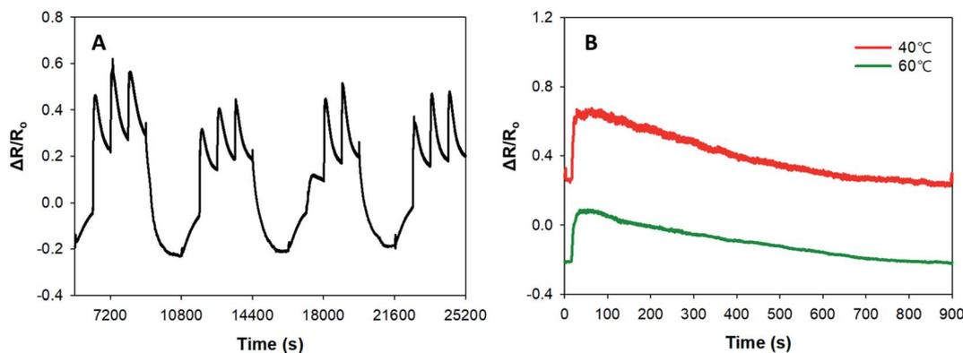
Fig. 8 (A) Repeatability and reversibility of the PPY-SEBS hybrid scaffold material in detecting NH<sub>3</sub> gas, (B) response and recovery time of the PPY-SEBS hybrid scaffold.
