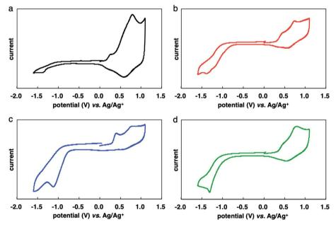
Fig. 4 Cyclic voltammograms of rr-P3HT (a: black), P(3HT-ran-uTIIa) (b: red), P(3HT-ran-uTIIb) (c: blue), and P(3HT-ran-uTIIc) (d: green). Conditions: electrolytic solution of 0.1 M  $Bu_4NBF_4/CH_3CN$ , working electrode: glassy carbon or ITO/PET, counter electrode: Pt, reference electrode: Ag/AgCl, scan rate: 100 mV s<sup>-1</sup>.
