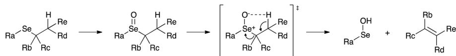
Scheme 4 Mechanistic details of selenoxide elimination leading to the formation of selenenic acid and olefin. Selenenic acid undergoes disproportionation and only seleninic acid was experimentally observed.
