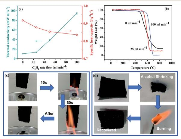
Fig. 4 Thermal conductivity and fire-resistance characterization of CNT sponges. (a) Thermal conductivity (T/C) coefficient and specific heat capacity curves for CNT sponges formed at  $C_2H_2$  flow rates of 0, 25, 50, and 100 mL min<sup>-1</sup>; (b) TG curves obtained in air for the CNT sponges formed at different  $C_2H_2$  flow rates; (c) vertical burning test of a CNT sponge; (d) photographs of a CNT sponge undergoing shrinking, burning, and recovering.
