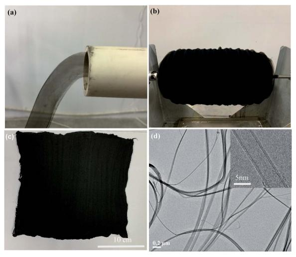
Fig. 2 Optical and TEM images of CNT assemblies. (a) A hollow cylindrical CNT assembly (HCCA) being extruded out from a reactor; (b) an LMCA winded on a winding drum; (c) an LMCA of  $\sim$ 10 mm thick taken off from the winding drum; (d) a TEM image of CNTs in HCCA (inset: HR-TEM image showing double-walled CNTs with a diameter of  $\sim$ 5 nm).
