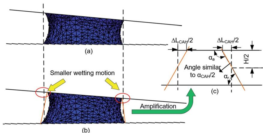
Fig. 6 Analysis about the CAH effect based on simulation (a) simulation result without CAH (b) simulation result with  $\alpha_{CAH} = 30^\circ$  (c) theoretical analysis model about the effect of  $\alpha_{CAH}$ .
