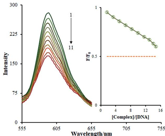
Fig. 6 The emission spectra of the DNA-EB system in the presence of increasing amounts (1 is lowest, 11 is highest) of the Ho(III) complex; inset: a plot of  $F/F_0$  versus  $[\text{Complex}]/[\text{DNA}]$ .
