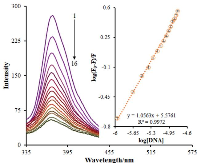
Fig. 5 The fluorescence spectra of complex-DNA; Ho(III) complex concentration:  $2.0 \times 10^{-5}$  M in Tris-buffer at pH 7.2; DNA concentrations (1 is lowest, 16 is highest): 0, 1.1, 2.2, 3.3, 4.4, 5.5, 6.6, 7.7, 8.8, 9.9, 11.0, 12.1, 13.2, 14.3, 15.4 and 16.5  $\mu\text{M}$ ; inset: plot of  $\log(F_0 - F)/F$  vs  $\log[\text{DNA}]$ .
