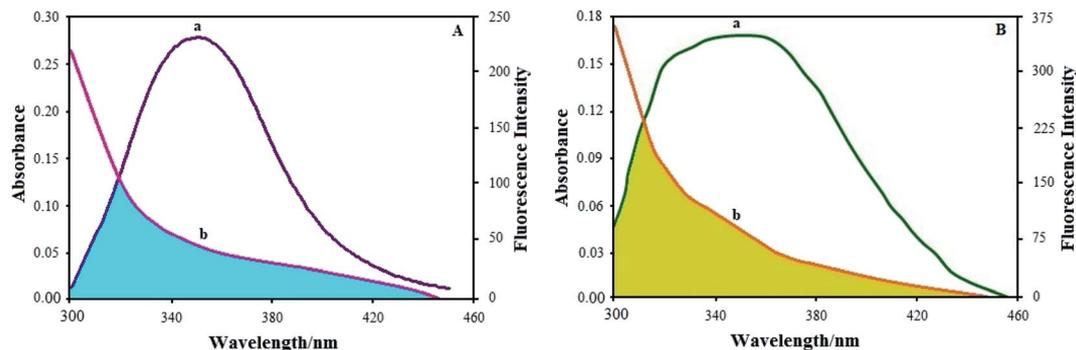
Fig. 11 (A) Overlap of the fluorescence spectrum of BSA ( $T = 298$  K) and the UV absorption spectrum of the Ho(III) complex: (a) fluorescence spectrum of BSA; (b) UV absorption spectrum of the Ho(III) complex. (B) Overlap of the fluorescence spectrum of HSA ( $T = 298$  K) and the UV absorption spectrum of the Ho(III) complex: (a) fluorescence spectrum of HSA; (b) UV absorption spectrum of the Ho(III) complex.
