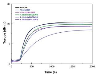
Fig. 7 Curing curves of the NR composites at 143 °C
