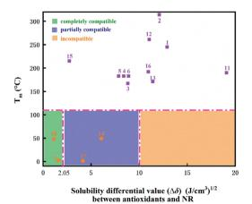
Fig. 3 The map shows 18 natural phenolic antioxidants with melting point  $T_{\rm m}$  and the solubility differential value ( $\Delta\delta$ ) between antioxidants and NR. The orange dots (no. 7, 14, 17, 18 samples) may be potential candidates according to  $\Delta\delta$  and  $T_{\rm m}$  values.
