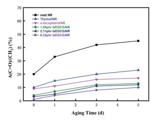
Fig. 11 The ratio of  $A_{\rm (C=O)}/A_{\rm (CH_2)}$  with different antioxidants/NR composites after thermo-oxidative aging times for 1, 3 and 5 days at 100 °C.
