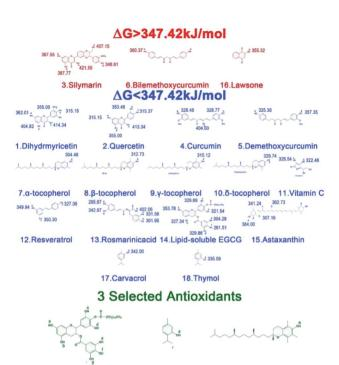
Fig. 4 Screening process of natural phenolic antioxidants and the  $\Delta G$  (kJ mol $^{-1}$ ) of ArO-H bonds at different position are indicated in the structures.
