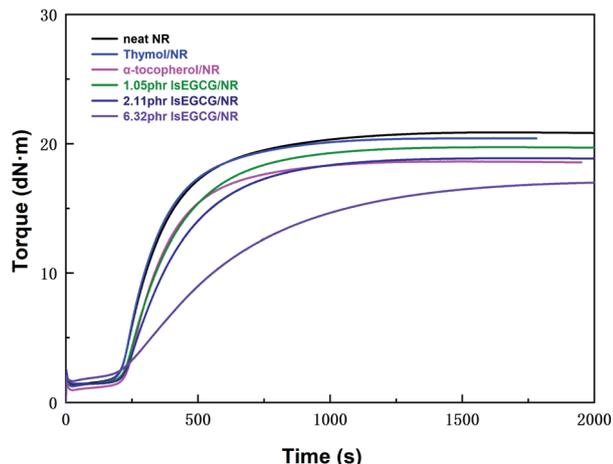
Fig. 7 Curing curves of the NR composites at 143 °C.
