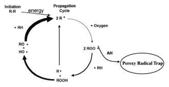
Fig. 2 Thermo-oxidative aging reaction of rubber (RH) in the presence of antioxidant (AH).
