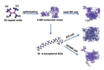
Fig. 1 Construction processes of the neat NR, AO (take  $\alpha$ -tocopherol as an example) and AO/NR amorphous cells (the magenta, blue and yellow represent C, H and O atoms, respectively).
