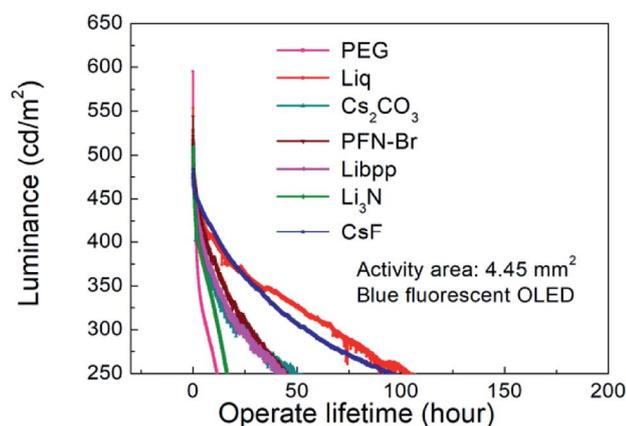
Fig. 4 The lifetime of the small-area blue fluorescent OLEDs with various interfacial materials.
