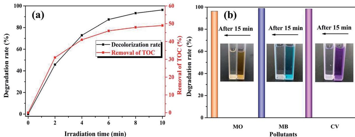
Fig. 6 (a) TOC removal of RhB, (b) the degradation of MO, MB, and CV ( $(\text{K-Fe}) = 1.0 \text{ g L}^{-1}$ ,  $\text{pH} = 7.2$ , (oxalic acid) = 1.0 mM,  $(\text{H}_2\text{O}_2) = 0.5 \text{ mM}$ , (organic dyes) = 100 mL,  $10 \text{ mg L}^{-1}$ ).
