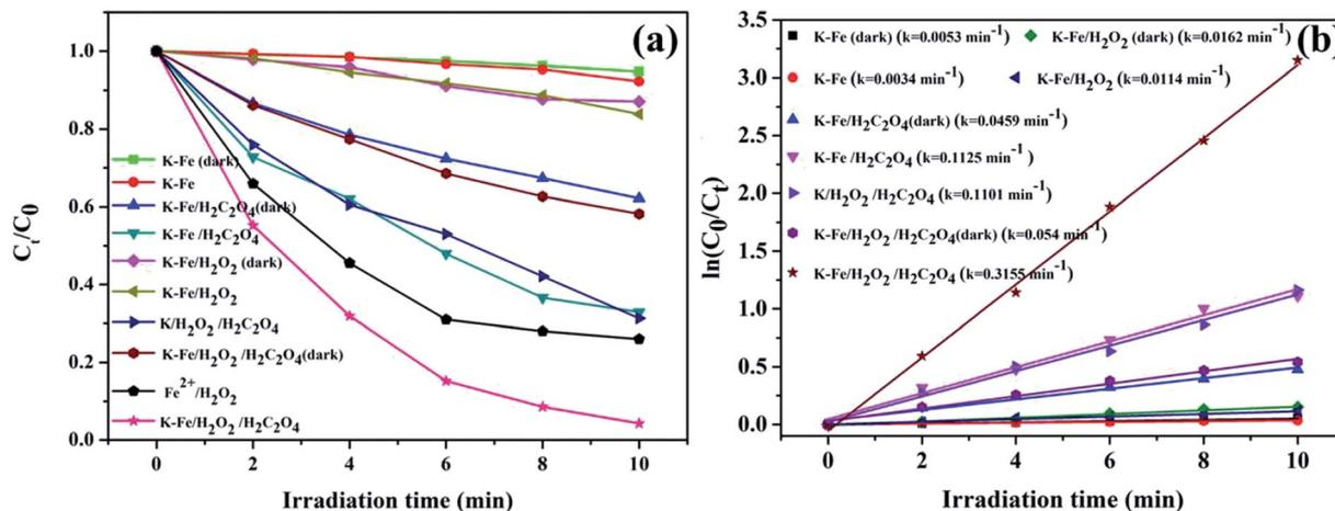
Fig. 4 (a) Degradation activity curves for RhB under different conditions, (b) kinetics for the degradation of RhB ((K-Fe) = 1.0 g L<sup>-1</sup>, pH = 7.2, (oxalic acid) = 1.0 mM, (H<sub>2</sub>O<sub>2</sub>) = 0.5 mM).
