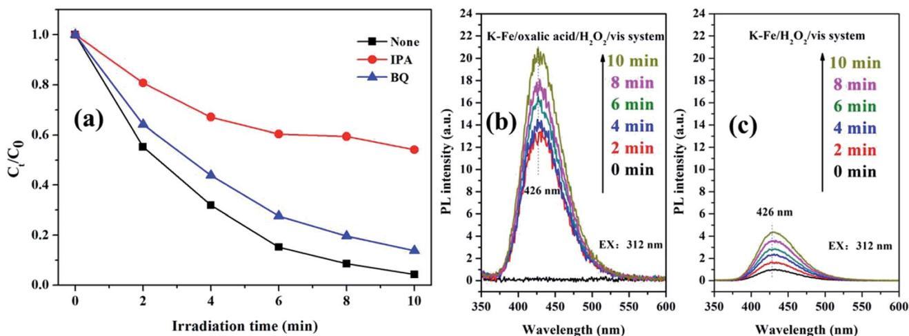
Fig. 9 (a) The trapping experiment with different scavengers added in the K-Fe/oxalic acid/ $\text{H}_2\text{O}_2$ /visible light system, (b)  $\cdot\text{OH}$ -trapping fluorescence spectra of the K-Fe/oxalic acid/ $\text{H}_2\text{O}_2$ /visible light system, (c)  $\cdot\text{OH}$ -trapping fluorescence spectra of the K-Fe/ $\text{H}_2\text{O}_2$ /visible light system.
