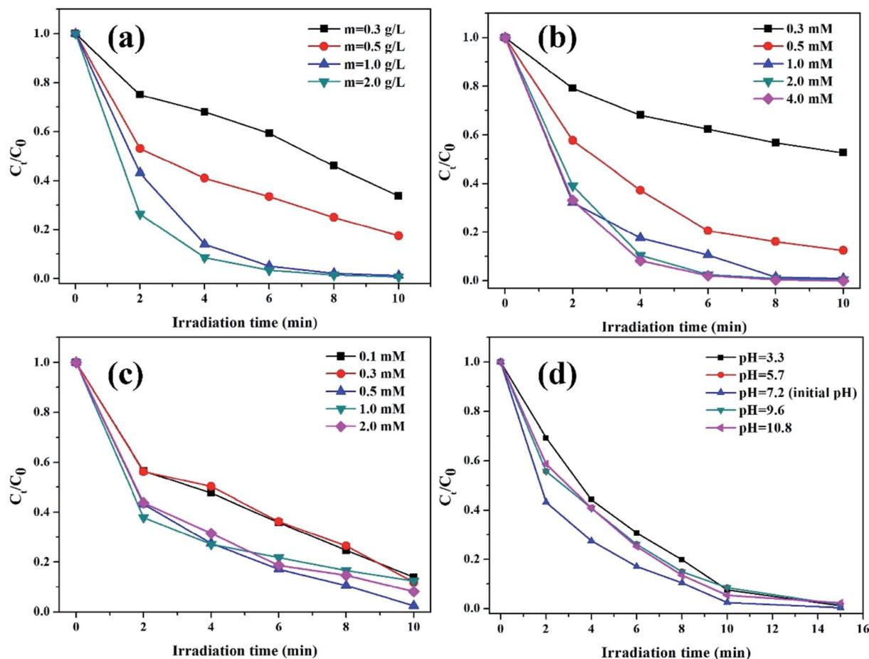
Fig. 5 (a) Effect of catalyst dosage (pH = 7.2, (oxalic acid) = 1.0 mM, ( $H_2O_2$ ) = 0.5 mM), (b) oxalic acid concentration ((K-Fe) = 1.0 g L<sup>-1</sup>, pH = 7.2, ( $H_2O_2$ ) = 0.5 mM), (c)  $H_2O_2$  concentration ((K-Fe) = 1.0 g L<sup>-1</sup>, pH = 7.2, (oxalic acid) = 1.0 mM), (d) initial pH ((K-Fe) = 1.0 g L<sup>-1</sup>, (oxalic acid) = 1.0 mM, ( $H_2O_2$ ) = 0.5 mM) on the degradation of RhB.
