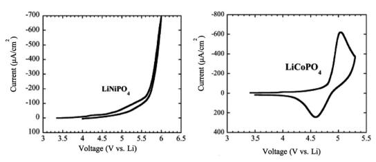
Fig. 14 Cyclic voltammetry of LiNiPO<sub>4</sub> and LiCoPO<sub>4</sub> at a scan rate of 0.2 mV s<sup>-1,135</sup>
