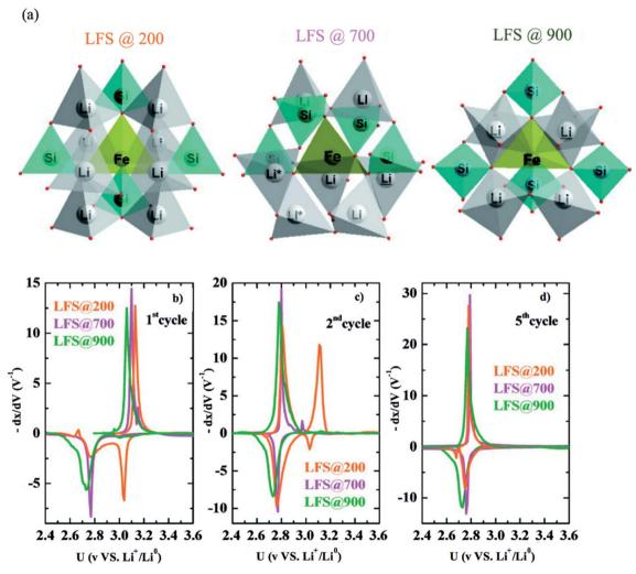
Fig. 15 (a) The three polymorphs of  $Li_2$ FeSiO<sub>4</sub>, derivative plots obtained from PITT measurements in the (b) first, (c) second, and (d) fifth cycles for all three polymorphs.<sup>141</sup>
