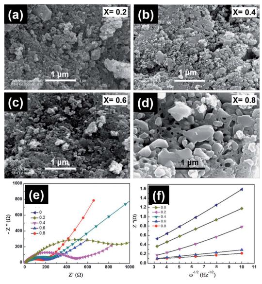
Fig. 13 (a–d) FESEM images, (e) impedance spectra, and (f) the relationship between Z'' and the square root of frequency ( $\omega^{-1/2}$ ) in the low-frequency region for LiMn<sub>1-x</sub>Fe<sub>x</sub>PO<sub>4</sub> at different compositions.<sup>131</sup>
