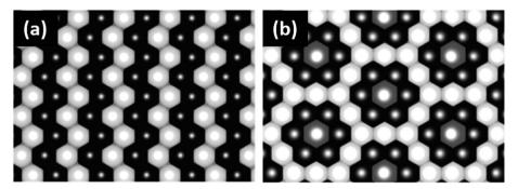
Fig. 7 (a) TM layer ordering of the flower structure and (b) transition metal layer ordering of the zigzag structure.<sup>59</sup>
