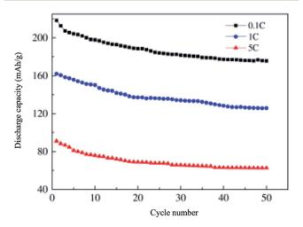
Fig. 17 Cyclic performance of nano C/Li<sub>2</sub>MnSiO<sub>4</sub> synthesized by ionothermal method, the material is tested in the potential range of 2.5-4.5 V.153
