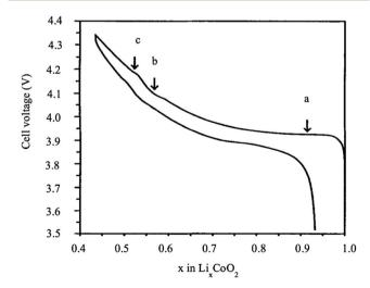
Fig. 3 Cell voltage of  $Li_xCoO_2$  as a function of x.<sup>12</sup>
