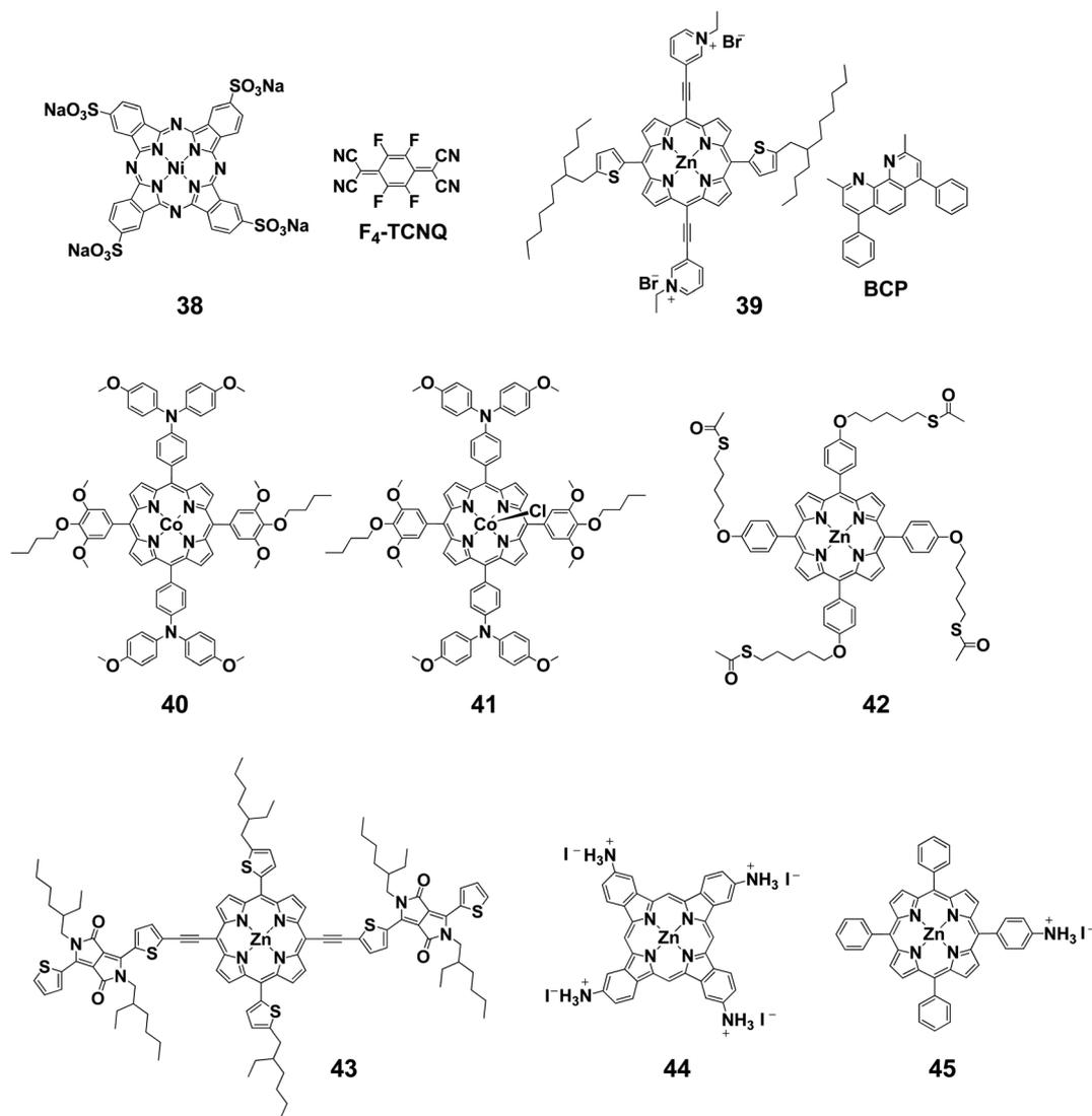
Fig. 2 Structures of porphyrins and phthalocyanines for interface engineering.
