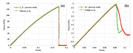
Fig. 2 Stress-strain curves of (a)  $C_3N$  nanosheets (in comparison with Shirazi<sup>30</sup>) and (b) pure aluminum (in comparison with Sedigh<sup>26</sup>).
