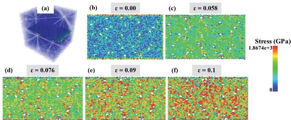
Fig. 7 Von Mises stress distribution of the (a) nanocomposite before the tensile test, (b)  $C_3N$  nanosheets when strain is  $\epsilon = 0$ , (c) when strain is  $\epsilon = 0.058$ , (d) when strain is  $\epsilon = 0.076$ , (e) when strain is  $\epsilon = 0.09$ , (f) when strain is  $\epsilon = 0.1$ .
