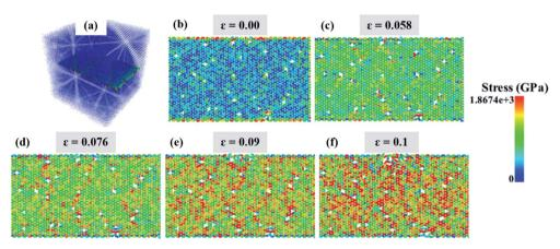
Fig. 7 Von Mises stress distribution of the (a) nanocomposite before the tensile test, (b)  $C_3N$  nanosheets when strain is  $\varepsilon = 0$ , (c) when strain is  $\varepsilon = 0.058$ , (d) when strain is  $\varepsilon = 0.076$ , (e) when strain is  $\varepsilon = 0.09$ , (f) when strain is  $\varepsilon = 0.18$ .
