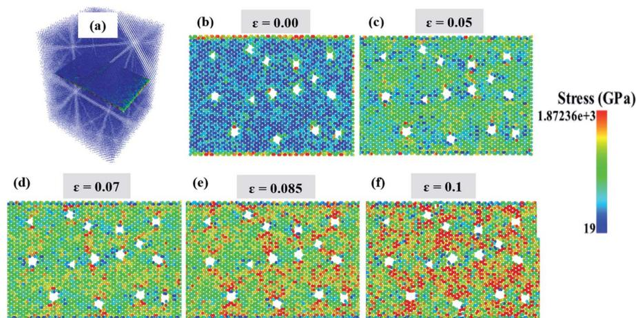
Fig. 11 (a) Initial configuration of the nanocomposite. (b to f) Stress distribution and concentration in the Al–C<sub>3</sub>N nanocomposites in the presence of 15 void defects at different strains after equilibrium (b)  $\epsilon = 0.0$ , (c)  $\epsilon = 0.05$ , (d)  $\epsilon = 0.07$ , (e)  $\epsilon = 0.085$  and (f)  $\epsilon = 0.1$  (at the beginning of the structure disruption).
