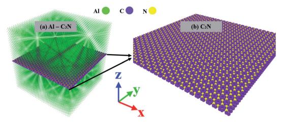
Fig. 1 The initial configuration in the present simulation consists of (a)  $Al-C_3N$  nanocomposite with 2.3 wt%  $C_3N$  embedded in the center of the aluminum plate. (b)  $C_3N$  monolayer. The aluminum, carbon, and nitrogen atoms are shown in green, purple, and yellow, respectively.
