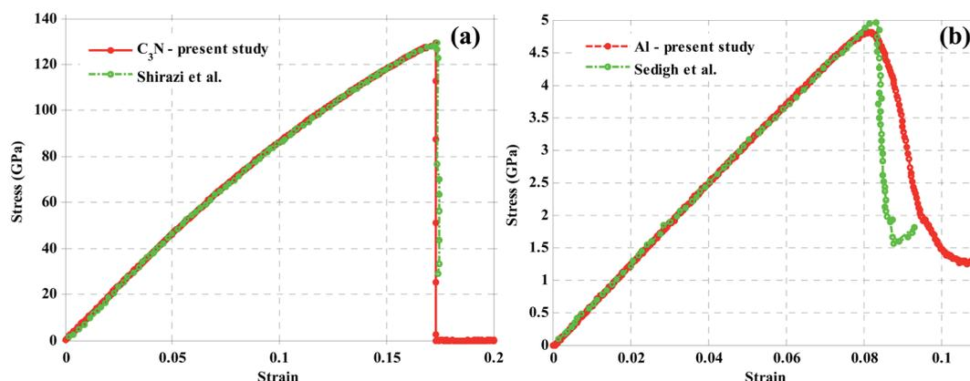
Fig. 2 Stress–strain curves of (a) C<sub>3</sub>N nanosheets (in comparison with Shirazi<sup>30</sup>) and (b) pure aluminum (in comparison with Sedigh<sup>26</sup>).
