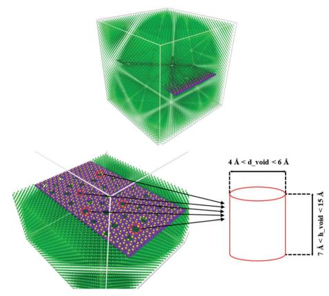
Fig. 9 Initial configuration of the Al- $C_3$ N nanocomposite in the presence of a cylindrical void defect with a diameter of 4 to 6 Å and a height of 7 to 15 Å in the interface between Al and the  $C_3$ N nanosheets.
