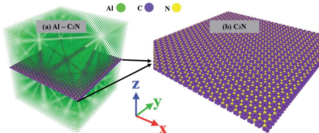
Fig. 1 The initial configuration in the present simulation consists of (a) Al–C<sub>3</sub>N nanocomposite with 2.3 wt% C<sub>3</sub>N embedded in the center of the aluminum plate. (b) C<sub>3</sub>N monolayer. The aluminum, carbon, and nitrogen atoms are shown in green, purple, and yellow, respectively.
