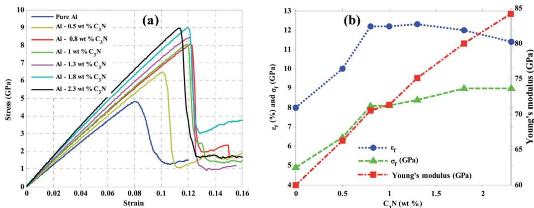
Fig. 3 (a) Stress–strain curve, and (b) the fracture strain and stress variations, as well as the Young's modulus of Al–C<sub>3</sub>N nanocomposites with different weight percentages of C<sub>3</sub>N as the filler at 300 K.
