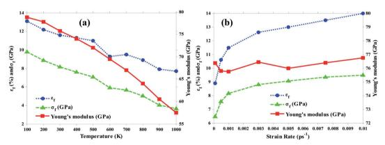
Fig. 4 Variation of Young's modulus, fracture strength and strain of nanocomposite with 1.3 wt%  $C_3N$  by (a) temperature rise and (b) strain rate increase
