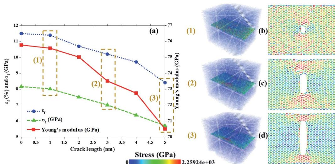
Fig. 8 (a) Changes of the Young's modulus, fracture strength and strain with increasing crack length in the Al- $C_3N$  nanocomposites. (b), (c) and (d) The stress distribution in the  $C_3N$  nanosheets in the presence of cracks with lengths of 1, 3, and 5 nm at the beginning of the disruption.
