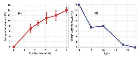
Fig. 13 (a) The energy changes adsorbed by the  $Al-C_3N$  nanocomposite. (b) The energy changes adsorbed by the nanocomposite by varying the  $C_3N$  nanoparticle positioning distance from the aluminum surface.
