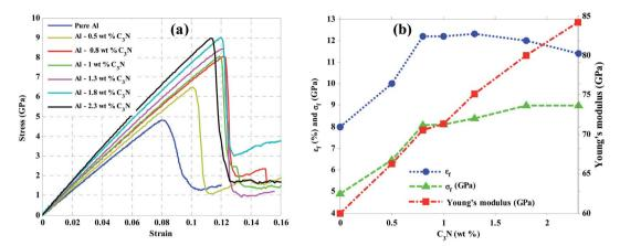
Fig. 3 (a) Stress-strain curve, and (b) the fracture strain and stress variations, as well as the Young's modulus of Al-  $C_3N$  nanocomposites with different weight percentages of  $C_3N$  as the filler at 300 K.
