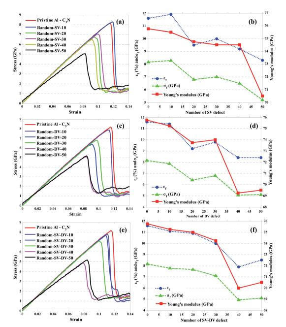
Fig. 6 (a), (b), and (c) The stress-strain curve of Al-  $C_3N$  nanocomposites in the presence of SV, DV and SV-DV defects, respectively, as a function of increasing the number of defects in the  $C_3N$  2D nanosheets. The Young's modulus, fracture strength, and strain are shown by increasing the number of defects for SV (d), DV (e), and SV-DV (f).
