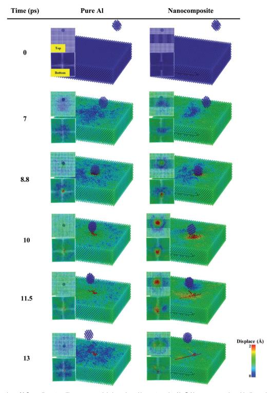
Fig. 12 Configuration of 1.8 nm diameter silicon nanoparticle launch and impact on the Al $-C_3N$  nanocomposite with dimensions of 12.5  $\times$  12.5  $\times$  2.4 nm along the angle (42°) concerning the yz plane at different times.
