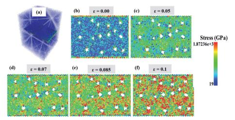
Fig. 11 (a) Initial configuration of the nanocomposite. (b to f) Stress distribution and concentration in the Al-C<sub>3</sub>N nanocomposites in the presence of 15 void defects at different strains after equilibrium (b)  $\varepsilon = 0.0$ , (c)  $\varepsilon = 0.05$ , (d)  $\varepsilon = 0.07$ , (e)  $\varepsilon = 0.085$  and (f)  $\varepsilon = 0.1$  (at the beginning of the structure disruption).
