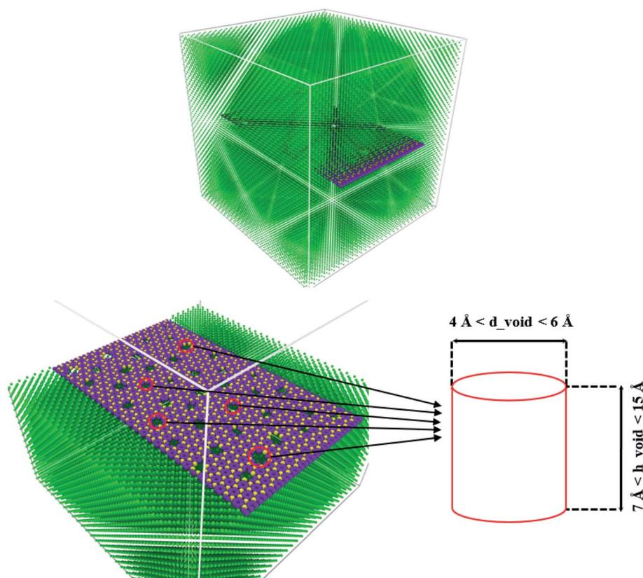
Fig. 9 Initial configuration of the Al–C<sub>3</sub>N nanocomposite in the presence of a cylindrical void defect with a diameter of 4 to 6 Å and a height of 7 to 15 Å in the interface between Al and the C<sub>3</sub>N nanosheets.
