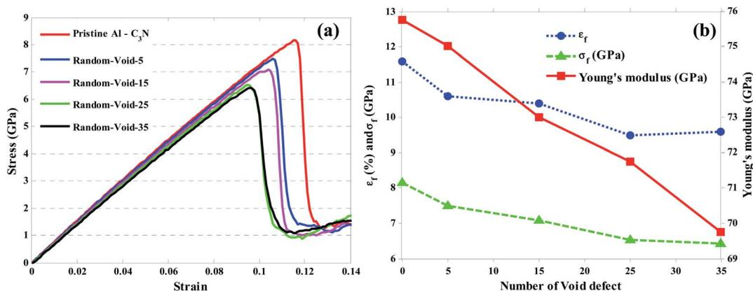
Fig. 10 (a) Stress–strain curve and (b) Young's modulus, fracture strength and strain of the Al–C<sub>3</sub>N nanocomposite with increasing void defect concentration.
