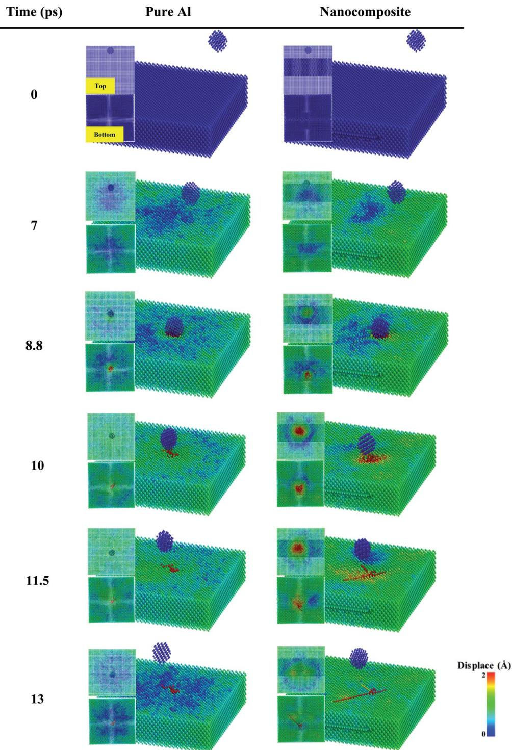
Fig. 12 Configuration of 1.8 nm diameter silicon nanoparticle launch and impact on the Al–C<sub>3</sub>N nanocomposite with dimensions of 12.5 × 12.5 × 2.4 nm along the angle (42°) concerning the yz plane at different times.
