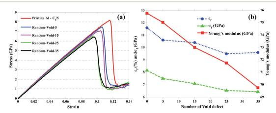
Fig. 10 (a) Stress-strain curve and (b) Young's modulus, fracture strength and strain of the Al-C<sub>3</sub>N nanocomposite with increasing void defect concentration.
