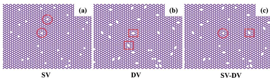
Fig. 5 The initial configuration of the C<sub>3</sub>N nanosheets containing (a) single vacancies (inside circles), (b) divacancies (inside squares) and (c) homogeneously both types.
