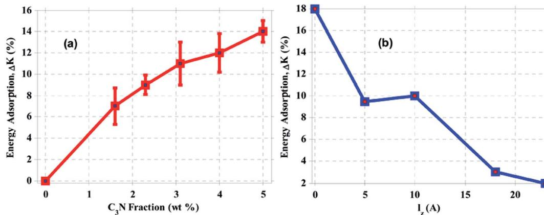
Fig. 13 (a) The energy changes adsorbed by the Al–C<sub>3</sub>N nanocomposite. (b) The energy changes adsorbed by the nanocomposite by varying the C<sub>3</sub>N nanoparticle positioning distance from the aluminum surface.
