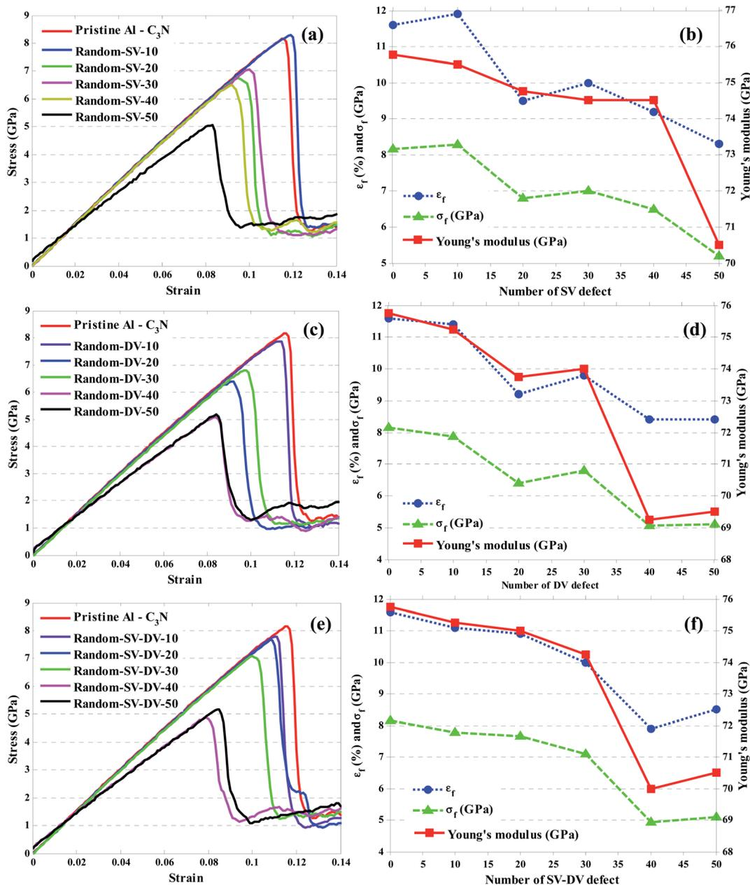
Fig. 6 (a), (b), and (c) The stress–strain curve of Al–C<sub>3</sub>N nanocomposites in the presence of SV, DV and SV–DV defects, respectively, as a function of increasing the number of defects in the C<sub>3</sub>N 2D nanosheets. The Young's modulus, fracture strength, and strain are shown by increasing the number of defects for SV (d), DV (e), and SV–DV (f).
