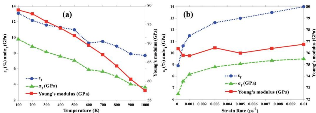
Fig. 4 Variation of Young's modulus, fracture strength and strain of nanocomposite with 1.3 wt% C<sub>3</sub>N by (a) temperature rise and (b) strain rate increase.
