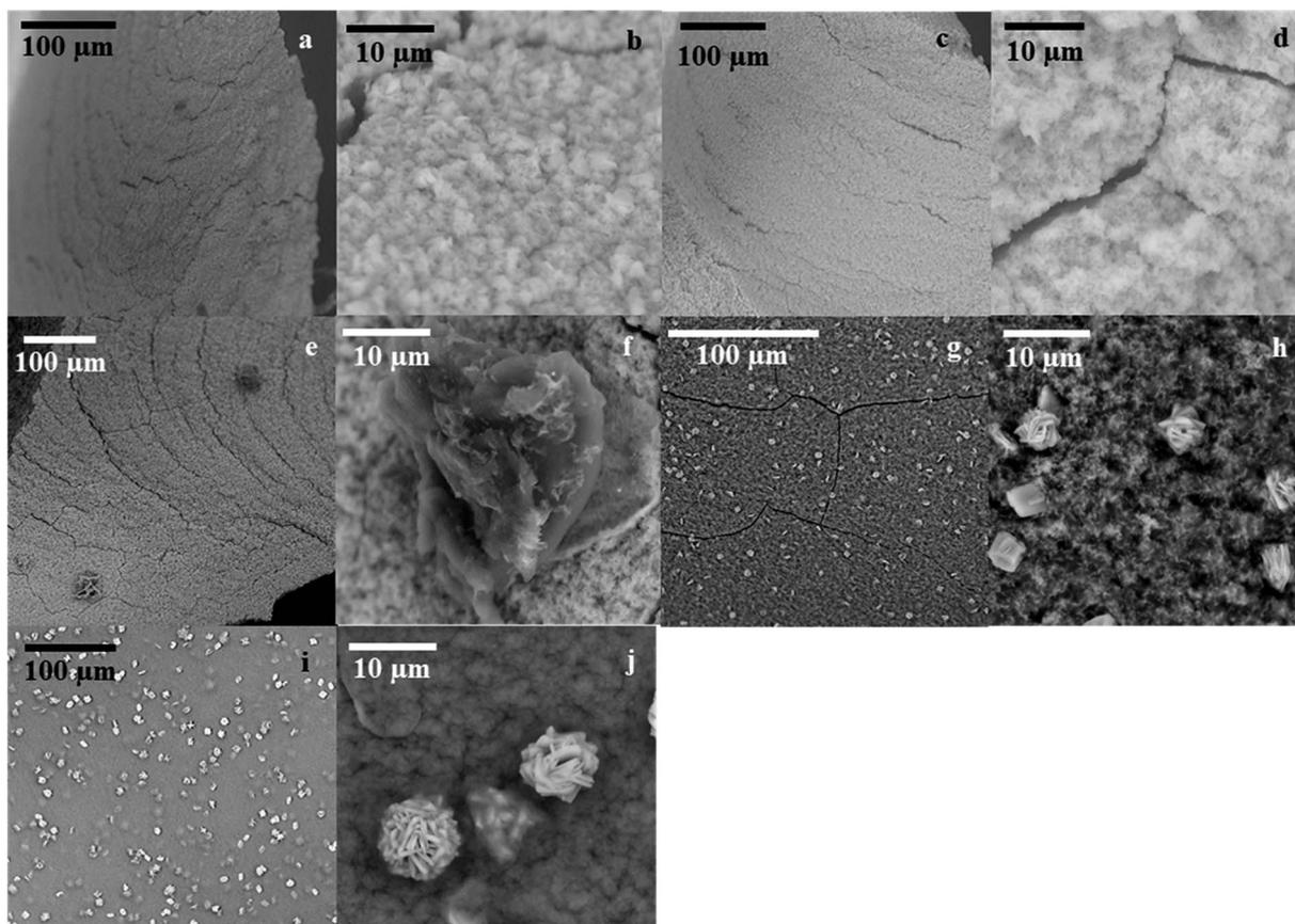
Fig. 2 SEM images of GcAPRD nanocrystal formed under various protein concentrations, (a and b) control (no enzyme), (c and d)  $0.02 \text{ mg mL}^{-1}$ , (e and f)  $0.10 \text{ mg mL}^{-1}$ , (g and h)  $0.50 \text{ mg mL}^{-1}$ , and (i and j)  $2.00 \text{ mg mL}^{-1}$ .
