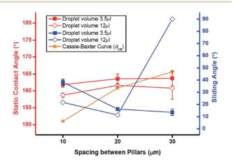
Fig. 4 Static contact angle (red lines, left axis) and sliding angle (blue lines, right axis) of samples with pillars height  $=10~\mu m$ . Orange line: prediction of Cassie–Baxter model.
