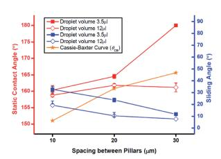
Fig. 3 Static contact angle (red lines, left axis) and sliding angle (blue lines, right axis) of samples with pillars with height  $=50~\mu m$ . Orange line: prediction of Cassie–Baxter model.
