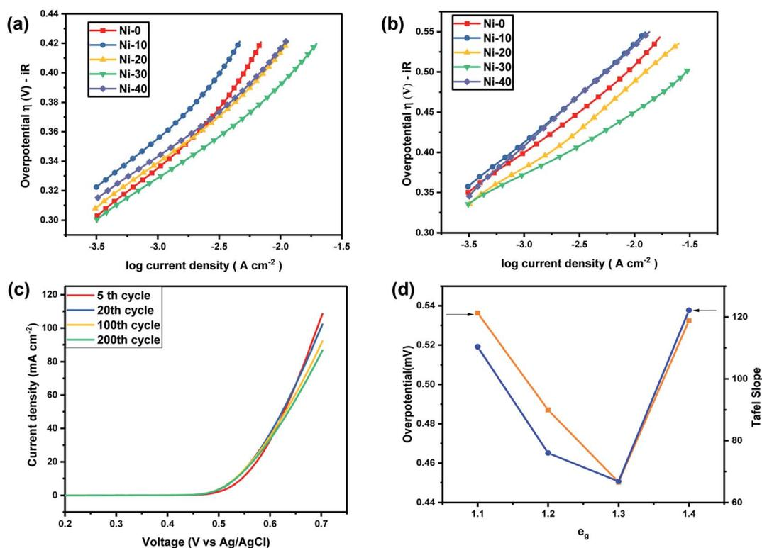
Fig. 7 (a) Tafel plot of  $\text{Ni}_x\text{Co}_{1-x}\text{O}$  at 5 M KOH. (b) Tafel plot of  $\text{Ni}_x\text{Co}_{1-x}\text{O}$  at 1 M KOH. (c) Showing stable OER activity of  $\text{Ni}_{0.3}\text{Co}_{0.7}\text{O}$  up to 200 cycles. (d) Volcano graph depicting correlation of  $e_g$  electrons with overpotential (at  $10 \text{ mA cm}^{-2}$ ) and the Tafel slope at 1 M KOH electrolyte.
