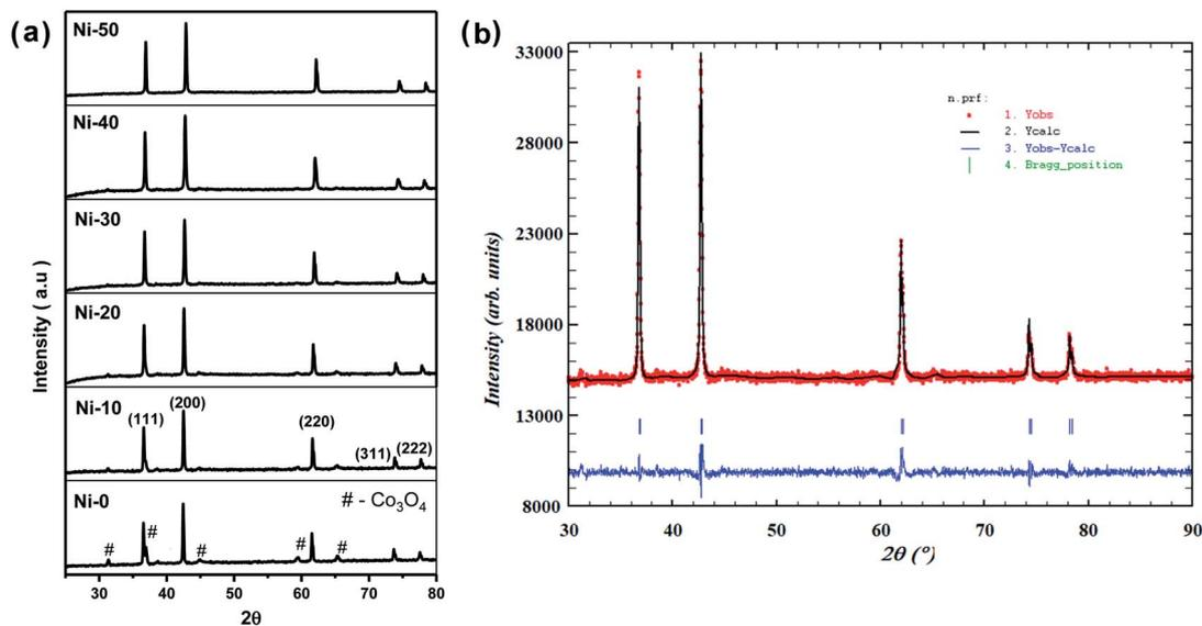
Fig. 1 (a) X-ray diffraction patterns of  $\text{Ni}_x\text{Co}_{1-x}\text{O}$  ( $x = 0, 0.1, 0.2, 0.3, 0.4, 0.5$ ) denoted as Ni-0 to Ni-50. (b) Rietveld refinement of XRD pattern of  $\text{Ni}_{0.3}\text{Co}_{0.7}\text{O}$ .
