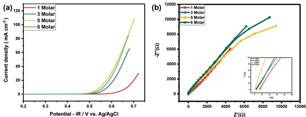
Fig. 5 (a) Variation of OER activity of  $\text{Ni}_{0.3}\text{Co}_{0.7}\text{O}$  with the concentration of electrolyte. (b) EIS measurement of  $\text{Ni}_{0.3}\text{Co}_{0.7}\text{O}$  for different concentration of electrolyte.
