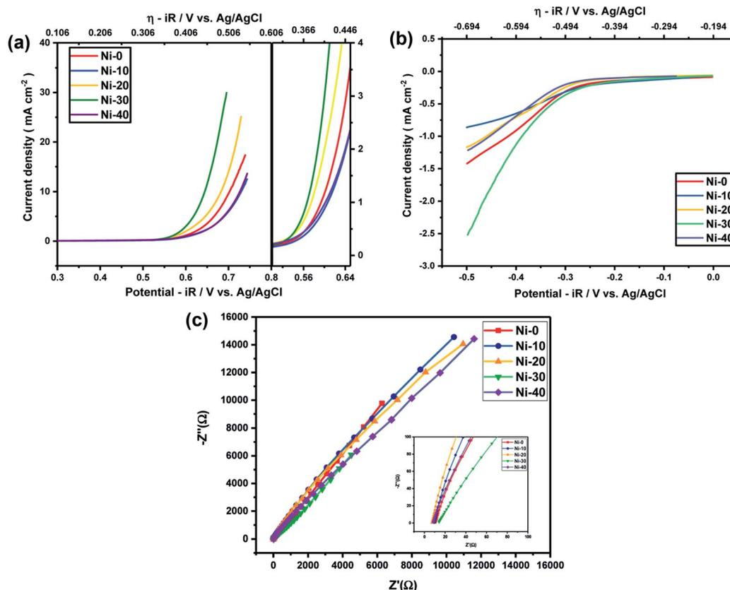
Fig. 4 (a) OER activity of  $\text{Ni}_x\text{Co}_{1-x}\text{O}$  at 1 M KOH electrolyte. (b) ORR activity of  $\text{Ni}_x\text{Co}_{1-x}\text{O}$  at 1 M KOH electrolyte. (c) EIS measurements of  $\text{Ni}_x\text{Co}_{1-x}\text{O}$  at 1 M KOH electrolyte.
