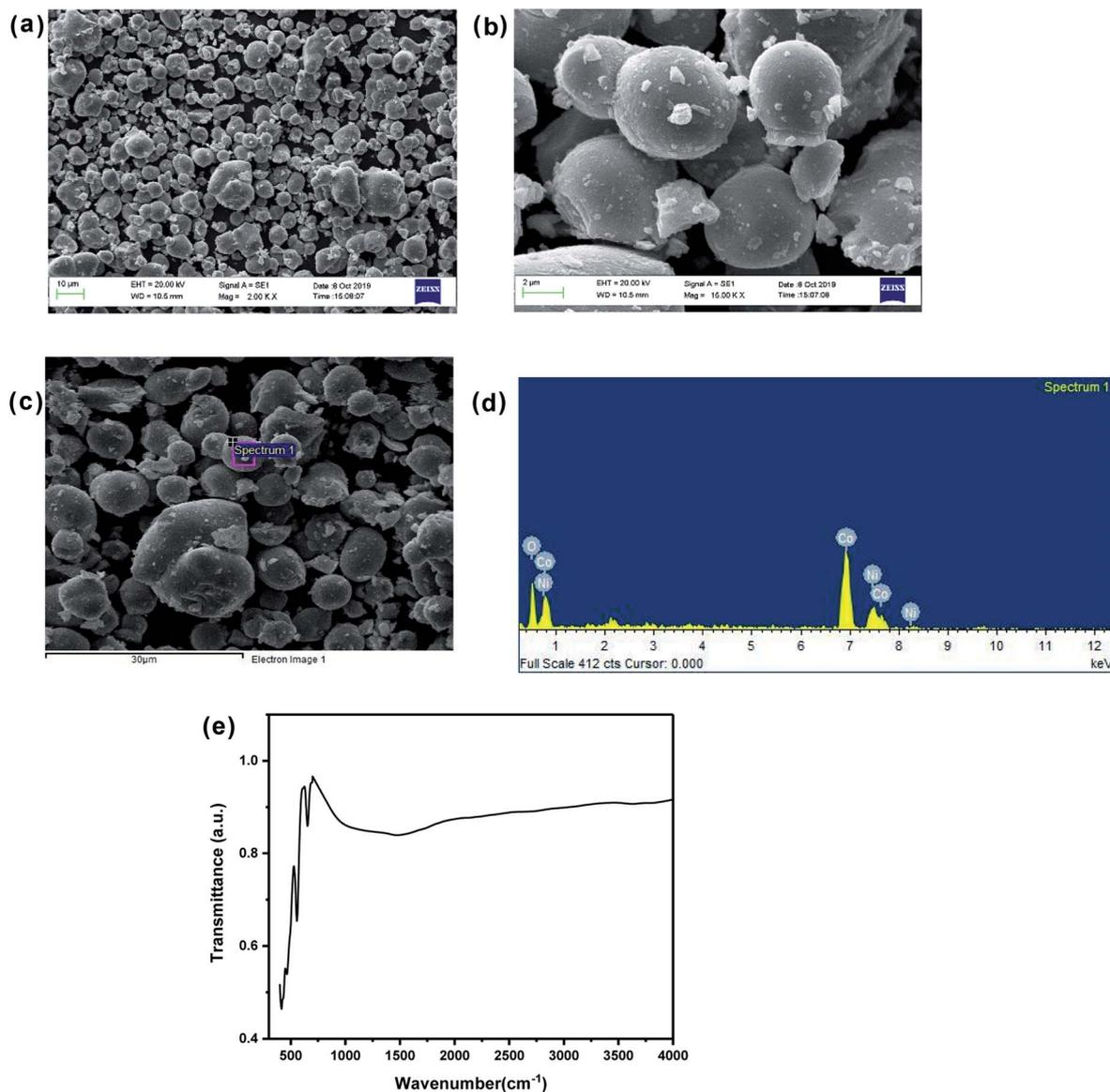
Fig. 2 (a) Scanning electron micrograph of  $\text{Ni}_{0.3}\text{Co}_{0.7}\text{O}$ . (b) Scanning electron micrograph (enlarged view) of  $\text{Ni}_{0.3}\text{Co}_{0.7}\text{O}$ . (c) Region selected for EDX spectra. (d) EDX analysis showing stoichiometric distribution of Co, Ni and O elements. (e) FTIR spectrum of  $\text{Ni}_{0.3}\text{Co}_{0.7}\text{O}$ .
