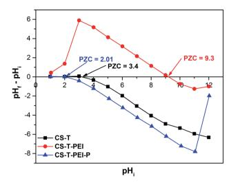
Fig. 4 Points of zero charge of CS-T, CS-T-PEI and CS-T-PEI-P.
