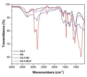
Fig. 2 FTIR spectra of CS-T, CS-T-PEI and CS-T-PEI-P.
