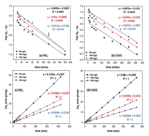
Fig. 6 Evolution in time of  $\log(q_{\rm e}-q_{\rm t})$  and  $t/q_{\rm t}$  for the pseudo-first order and pseudo-second order kinetics of NO<sub>3</sub><sup>-</sup> (a and c) and Cr(vi) (b and d) ions adsorption onto CS-T-PEI-P ( $m_{\rm ads}=0.2$  g, initial pH, 300 rpm, V = 50 mL and 23 °C).
