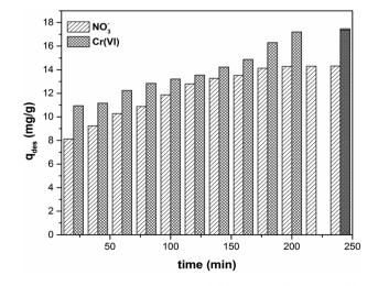
Fig. 7 Desorption of  $NO_3^-$  and  $Cr(v_i)$  from CS-T-PEI-P ( $C_i = 100 \text{ mg L}^{-1}$ , V = 50 mL,  $m_{\rm ads} = 0.2 \text{ g}$ , initial pH, RT, 300 rpm).
