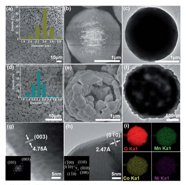
Fig. 2 (a–c) Typical SEM and TEM images of  $Ni_{1/3}Co_{1/3}Mn_{1/3}CO_3$  (inset: size distribution histograms derived from one hundred particles in (a)). (d–f) Typical SEM and TEM images of YS-NCM (inset: size distribution histograms gathered from one hundred particles in (d)). HRTEM images of (g) lateral plane and (h) frontal plane of YS-NCM (inset: fast Fourier transform (FFT) pattern). (i) EDS elemental mappings of YS-NCM.
