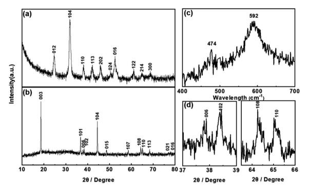
Fig. 3 XRD patterns of (a)  $Ni_{1/3}Co_{1/3}Mn_{1/3}CO_3$ , (b and d) YS-NCM. (c) Raman spectrum of YS-NCM.
