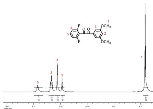
Fig. 1  $^1\text{H-NMR}$  spectrum of DFDMED in  $\text{DMSO-d}_6$ .
