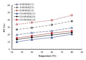
Fig. 7 Temperature dependence of WU for the crosslinkable and crosslinked membranes.
