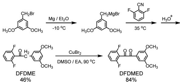
Scheme 1 Synthesis of the difluoro aromatic monomer DFDMED.
