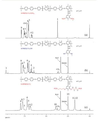
Fig. 3  $^{1}$ H NMR spectra of S-PAES(1/1)-OCH<sub>3</sub>, S-PAES(1/1)-OH, and S-SPAES(1/1).
