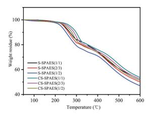
Fig. 9 TGA curves of the crosslinkable and crosslinked membranes.
