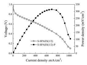
Fig. 11 Polarization (open symbols) and power density (solid symbols) curves of the single cell based on S-SPAES(1/2) membranes at  $60\,^{\circ}$ C in 100% RH condition.
