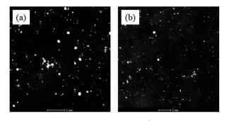
Fig. 4 TEM images of the membranes in Ag<sup>+</sup> forms. (a) S-SPAES(1/1), (b) CS-SPAES(1/1).
