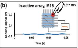
Fig. 8 (a) Dynamic voltage response for active sensing array ( $M_{33}$ ) against the external pressure of 0.0175 MPa. (b) Device showed negligible response, when the pressure is applied across in-active sensing array ( $M_{15}$ ).
