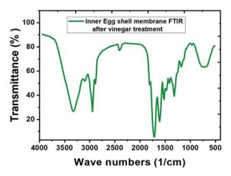
Fig. 4 FTIR spectra of IESM after the vinegar treatment to remove the egg outer shell.
