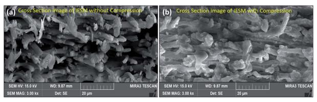
Cross-sectional SEM image of IESM in (a) normal and (b) compressed state.
