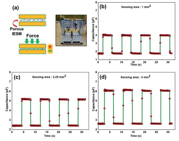
Fig. 7 (a) Schematics of the IESM based capacitive pressure sensor with and without applied pressure. The inset shows the photograph of linear servo motor. Capacitive change against sensing areas of (b) 1 mm<sup>2</sup>, (c) 2.25 mm<sup>2</sup>, and (d) 4 mm<sup>2</sup>, respectively.
