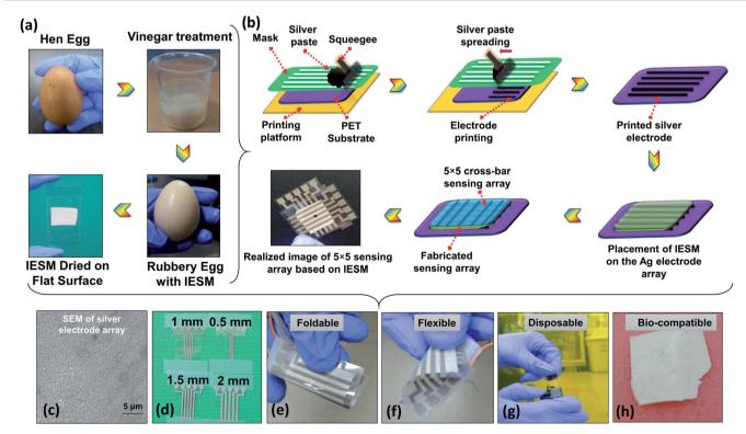
Fig. 1 Illustration of IESM based pressure sensor. (a) Processing of IESM using white vinegar. (b) Typical screen-printing (screen printer: AMX-1240M) of the  $5 \times 5$  electrode array. (c) SEM image of screen-printed silver electrodes. (d) Fabricated screen-printed silver electrode array on PET substrate having the width 0.5, 1, 1.5, and 2 mm respectively. The IESM based pressure sensor is: (e) foldable, (f) flexible, (g) disposable, and (h) biocompatible.
