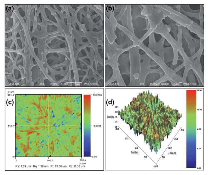
Fig. 2 Analysis of the IESM used in the capacitive and self-powered piezoelectric pressure sensor. (a) FESEM image of IESM at 10  $\mu$ m scaling. (b) FESEM image of IESM at 1  $\mu$ m scaling. (c) 2D nano profile of IESM.
