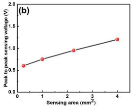
Fig. 5 (a) Capacitive change against the various sensing areas. It is shown that, the capacitance increases with increasing sensing area. (b) Peak to peak sensing voltage against various sensing areas. It is shown that, the voltage increases with increasing sensing area.
