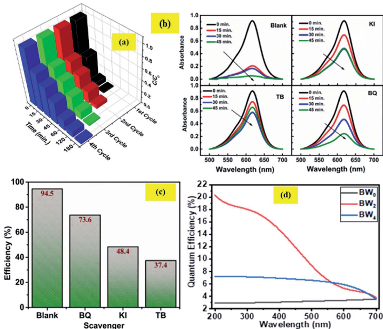
Fig. 11 (a) Cyclic tests of photodegradation of MG on BW<sub>2</sub> hybrid nanosheets. (b) Absorption spectra of MG dye with BW<sub>2</sub> photocatalyst in the presence of various scavengers (BQ, TB, and KI). (c) Effect of various scavengers in the photodegradation process of MG over BW<sub>2</sub> nanosheet hybrid and (d) IPCE spectra of BW<sub>0</sub>, BW<sub>2</sub>, and BW<sub>4</sub> hybrid nanosheets recorded at 0 V vs. Ag/AgCl in the wavelength range 200–700 nm.
