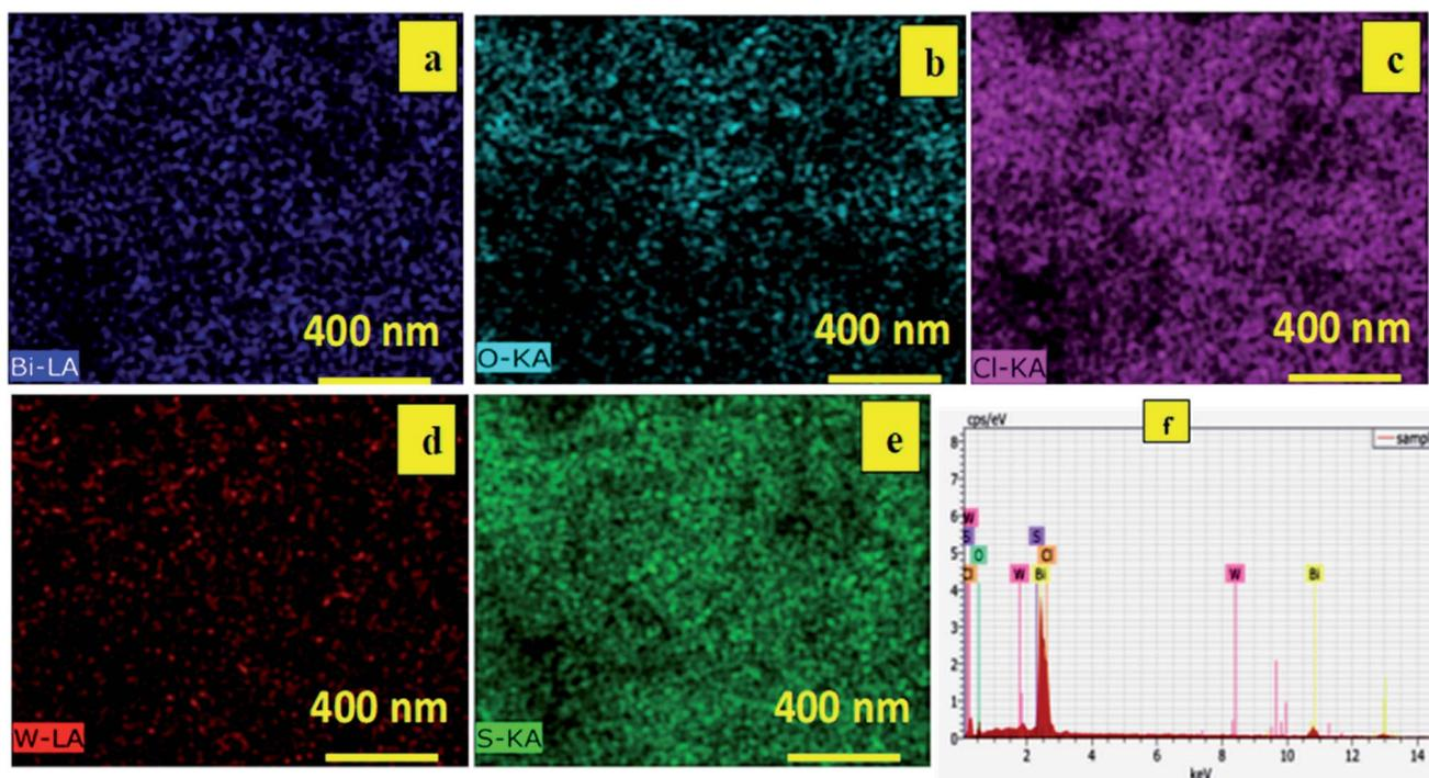
Fig. 3 Elemental mapping of Bi, O, Cl, W and S on the  $BW_2$  nanosheets showing (a) blue, (b) aqua, (c) magenta (d) red (e) green, corresponding to bismuth, oxygen, chlorine, tungsten, and sulphur, respectively and (f) EDX spectra of  $BW_2$  nanosheets.
