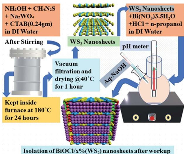
Fig. 1 Schematic diagram of the synthesis of BW<sub>X</sub> (X varies from 0% to 5%) hybrid nanosheets.
