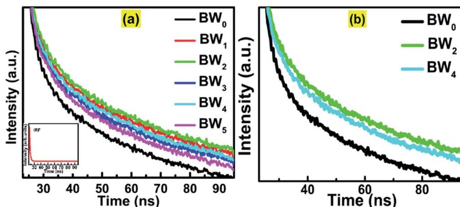
Fig. 8 (a) Time-correlated single-photon counting (TCSPC) spectra of  $BW_X$  hybrid nanosheets where  $X$  varies from 0% to 5%. Inset shows the IRF data. (b) Magnified TCSPC spectra for  $BW_0$ ,  $BW_2$  and  $BW_4$  nanosheets.
