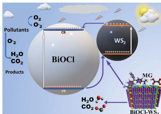
Fig. 12 Schematic diagram of photocatalysis mechanism.
