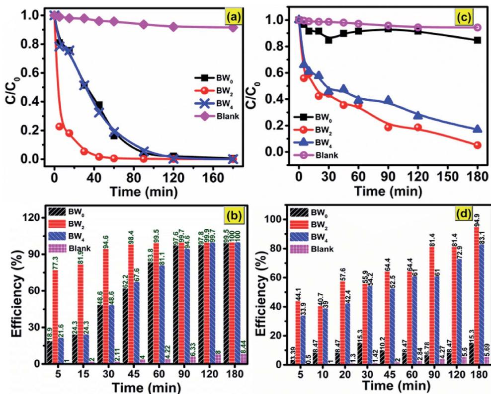
Fig. 9 Photocatalytic degradation of (a) MG dye; (c) Cr(vi) without catalyst and in the presence of BW<sub>0</sub>, BW<sub>2</sub>, and BW<sub>4</sub> under visible light irradiation; photocatalytic efficiency vs. time plot for (b) MG dye and (d) Cr(vi), over BW<sub>0</sub>, BW<sub>2</sub>, and BW<sub>4</sub> hybrid nanosheets.
