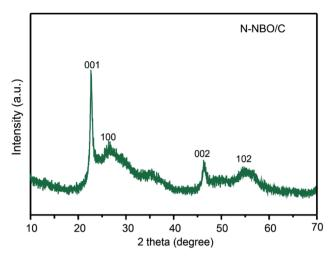
Fig. 9 XRD pattern of N-NBO/C after the photodegradation durability test (5 cycles).
