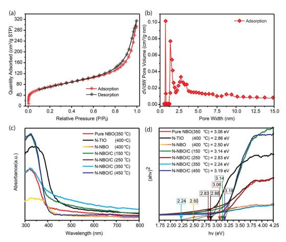
Fig. 4 N<sub>2</sub> adsorption-desorption isotherms of N-NBO/C, (b) pore size distribution curve, (c) UV-vis diffuse reflectance spectra of the asfabricated N-NBO/C at various calcination temperatures (150 °C, 250 °C, 350 °C and 450 °C) and pure NBO, and (d) plots of (αhv)² versus (hv).
