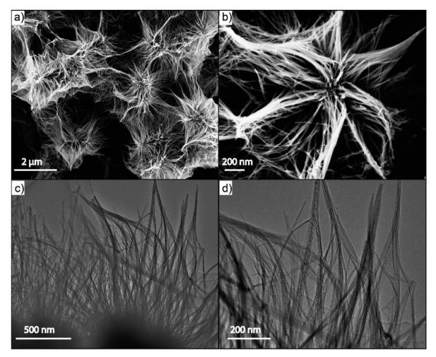
(a and c) Representative SEM and TEM images, and (b and d) magnified SEM and TEM images of N-NBO/C nanostructures, respectively.
