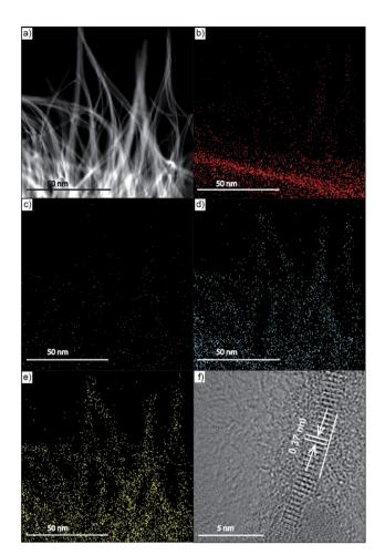
Fig. 3 (a-e) TEM image of as-prepared N-NBO/C and parallel EDS mapping images of C, N, Nb, and O, respectively. (f) HRTEM of the individual single wire N-NBO/C nanostructure.
