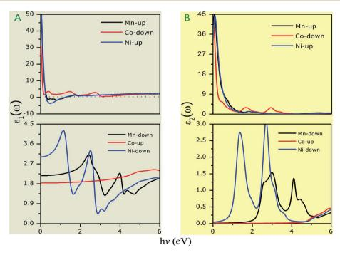
Fig. 7 Variation in dielectric constant with photon energy. (A) Real part ( $\epsilon_1$ ) with gray background and (B) imaginary part ( $\epsilon_1$ ) with yellowish background.
