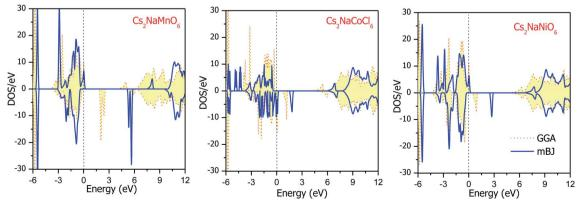
Fig. 4 Energy state distribution over the energy range of -6 to 12 eV by GGA and mBJ approximations.
