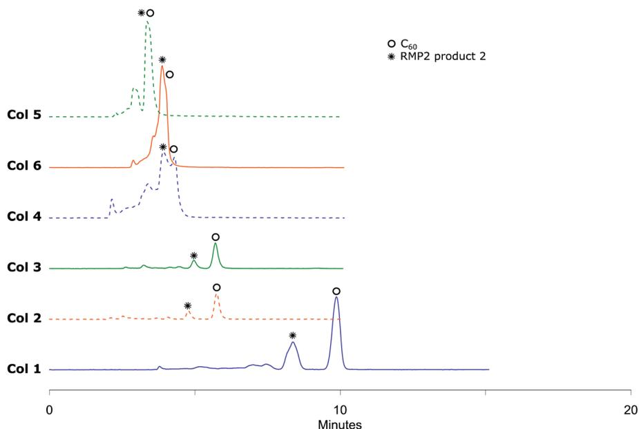
**Fig. 5** RPM2 chromatograms obtained by eluting with 45% (v/v) acetonitrile in toluene at 285 nm UV detection where Col 1, Col 2 and Col 3 show very good separation in short analysis time, Col 4, Col 5 and Col 6 does not separate RPM2 product **2**, neither from bis, tris and polyadducts nor from unreacted  $C_{60}$ .
