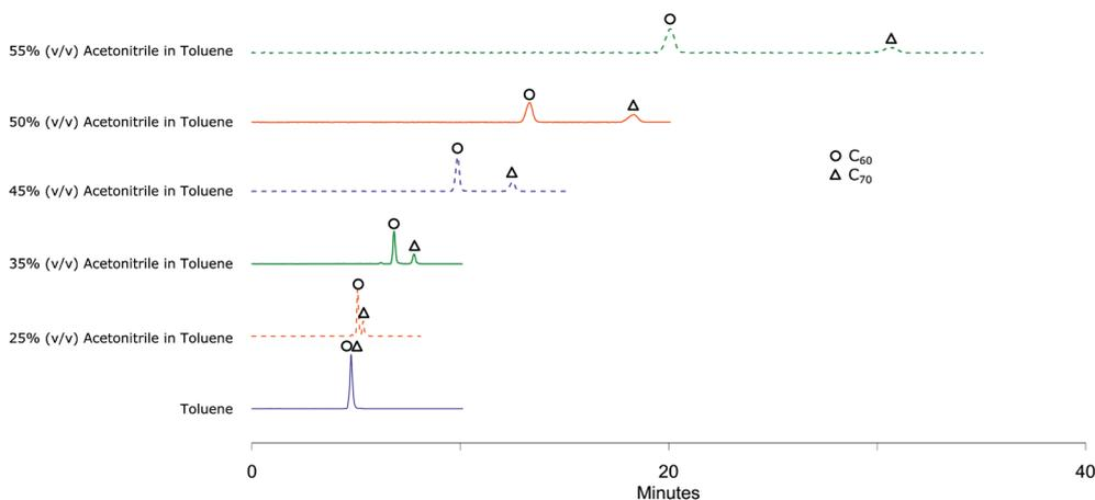
Fig. 1  $\text{C}_{60} + \text{C}_{70}$  mixture chromatograms obtained by eluting with  $1 \text{ mL min}^{-1}$  from Col 1 at 350 nm UV detection showing no separation in toluene, moderate separation in 25% (v/v) acetonitrile in toluene, very good separation in all other mobile phase compositions.
