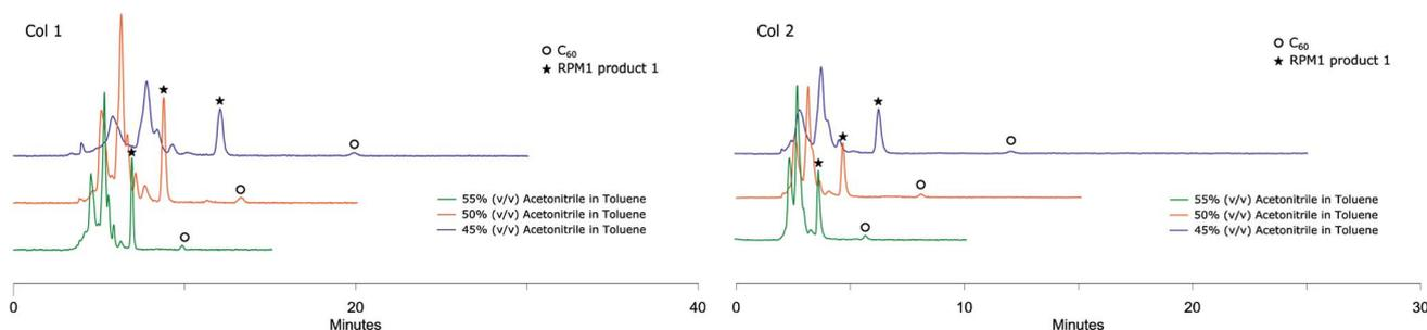
**Fig. 3** RPM1 chromatograms obtained by Col 1 and Col 2 eluting with different mobile phases, detection at 285 nm, both columns showing excellent separation of RPM1 product **1** from other components of the mixture.
