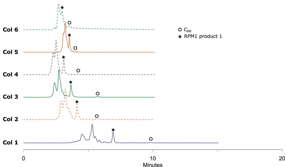
**Fig. 2** RPM1 chromatograms obtained by eluting with 45% (v/v) acetonitrile in toluene at 285 nm UV detection where Col 1, Col 2 and Col 3 show very good separation in a short analysis time, Col 4 shows moderate separation and Col 5 and Col 6 does not separate RPM1 product **1** from bis, tris and polyadducts and almost no separation from unreacted  $C_{60}$ .
