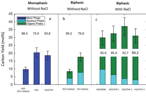
Fig. 4 The overall carbon yield (5-HMF and LA) under (a) monophasic, NaCl free reaction conditions, (b) biphasic (MIBK/H<sub>2</sub>O) solvent system without NaCl and (c) biphasic solvent system with NaCl inclusion. The numeric values in the illustration give the product ratio (in %)  $n_{5\text{-HMF}}/(n_{5\text{-HMF}} + n_{1\text{A}})$ . Biomass 6 g, BM/solvent ratio 1/16 (w/w).
