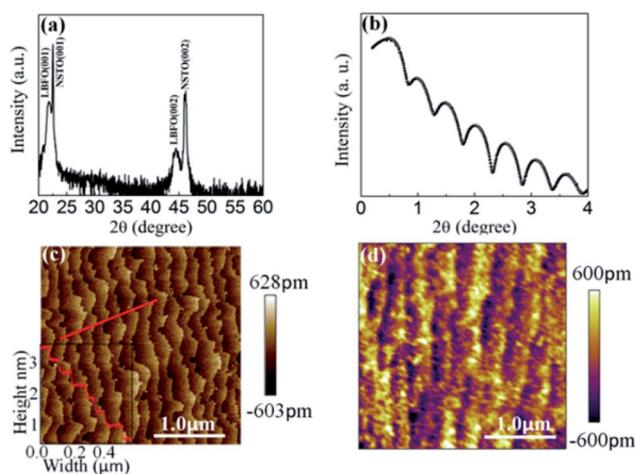
Fig. 1 (a) XRD  $\theta$ - $2\theta$  scan of the LBFO/NSTO (001) heterostructure. (b) X-ray reflectivity (XRR) measurements of the LBFO film. (c) Morphology of the etched NSTO. (d) Surface morphology of the 6.2 nm-thick LBFO layer grown on an NSTO substrate.
