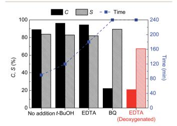
Fig. 5 Effect of scavengers in the photocatalytic performance of GCN-UL under air (black columns) and argon (red columns) atmospheres, using a UV-LED radiation source. The *C* and *S* values are determined to the maximum of AAD production, with the indication of the respective reaction time (•).
