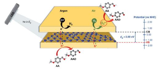
Scheme 1 Diagram of photocatalytic conversion of AA into AAD under deoxygenated and oxygenated conditions, using GCN-UL as photocatalyst and UV-LED as light source.
