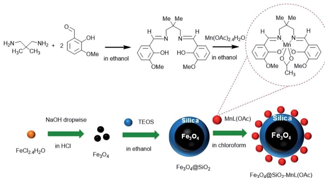
Scheme 1 Schematic of the preparation of Fe<sub>3</sub>O<sub>4</sub>@SiO<sub>2</sub>-[MnL(OAc)].
