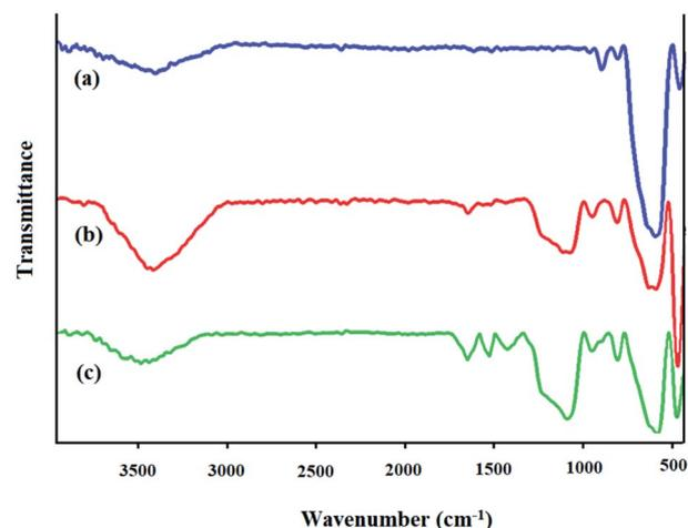
Fig. 2 FTIR spectra of (a) Fe<sub>3</sub>O<sub>4</sub>, (b) Fe<sub>3</sub>O<sub>4</sub>@SiO<sub>2</sub>, and (c) Fe<sub>3</sub>O<sub>4</sub>@SiO<sub>2</sub>-[MnL(OAc)].
