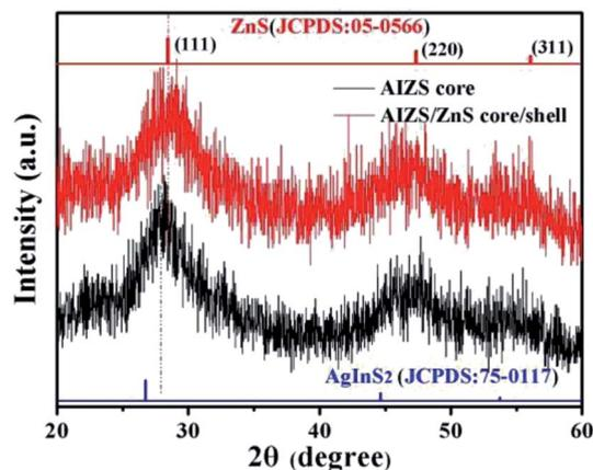
Fig. 1 XRD patterns of AIZS core and 1 monolayer AIZS/ZnS core/shell QDs (Ag : In : Zn = 1 : 4 : 1). Bulk main reflexes for ZnS (JCPDS #05-0566) and AgInS<sub>2</sub> (JCPDS #75-0117) are presented by line spectra.
