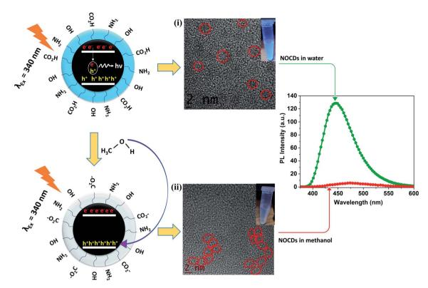
Schematic representation of PL quenching mechanism (i) NOCDs in water and (ii) NOCDs in methanol.
