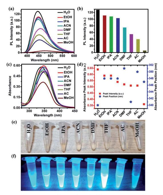
Fig. 2 Fluorescence of NOCDs in different solvents (a) PL spectra ( $\lambda_{ex} = 340$  nm) (b) variation in PL peak intensity (taken from (a)), (c) UV-vis absorption spectra, (d) peak absorption of NOCDs in different solvents, (e) photographs of NOCDs in different solvents under daylight and (f) NOCDs in different solvents irradiated by UV lamp ( $\lambda_{ex} = 365$  nm).
