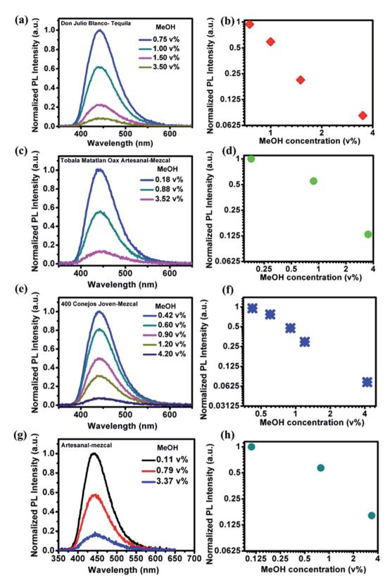
Fig. 6 Fluorescence response of NOCDs (measured at  $\lambda_{ex} = 340$  nm) in the presence of some tested spiked branded and unbranded alcoholic beverages after dilution (a and b) Don Julio Blanco-Tequila (tDJB), (c and d) Tobala Matatlan Oax Artesanal (traditional branded)-Mezcal (mTMOA), (e and f) 400 Conejos Joven-Mezcal (m400CJ) and (g and h) (traditional unbranded) Artesanal mezcal (mAR).
