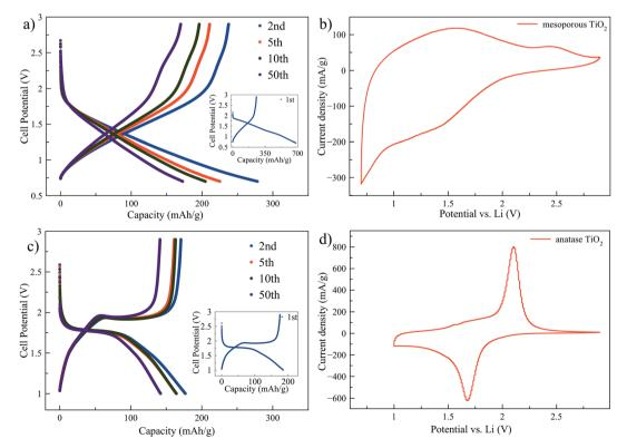
Fig. 1 Charge/discharge curves of mesoporous titania electrodes between 2.9 V and 0.7 V (a) and anatase titania electrodes between 2.9 V and 1 V (c) both cycled at 0.5C. Cyclic voltammetry curves ( $10^{th}$  cycle) scanned between 2.9 V and 0.7 V for mesoporous titania (b) and scanned between 2.9 V and 1 V for anatase (d) at scan rate 0.3 mV s<sup>-1</sup>.
