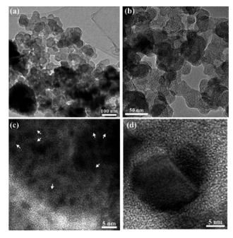
Fig. 6 Bright field TEM images of the electrode cycled to 1.7 V showing the overall morphology of the sample (a and b) and HR-TEM images showing the nanocrystalline anatase (c) and  $LiTiO_2$  (d).
