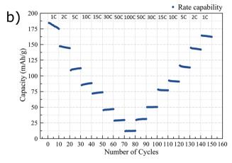
Fig. 3 Charge and discharge capacity vs. number of cycles, cycled at 0.5C (a) and the performance at higher rates (b) of the mesoporous titania electrodes.
