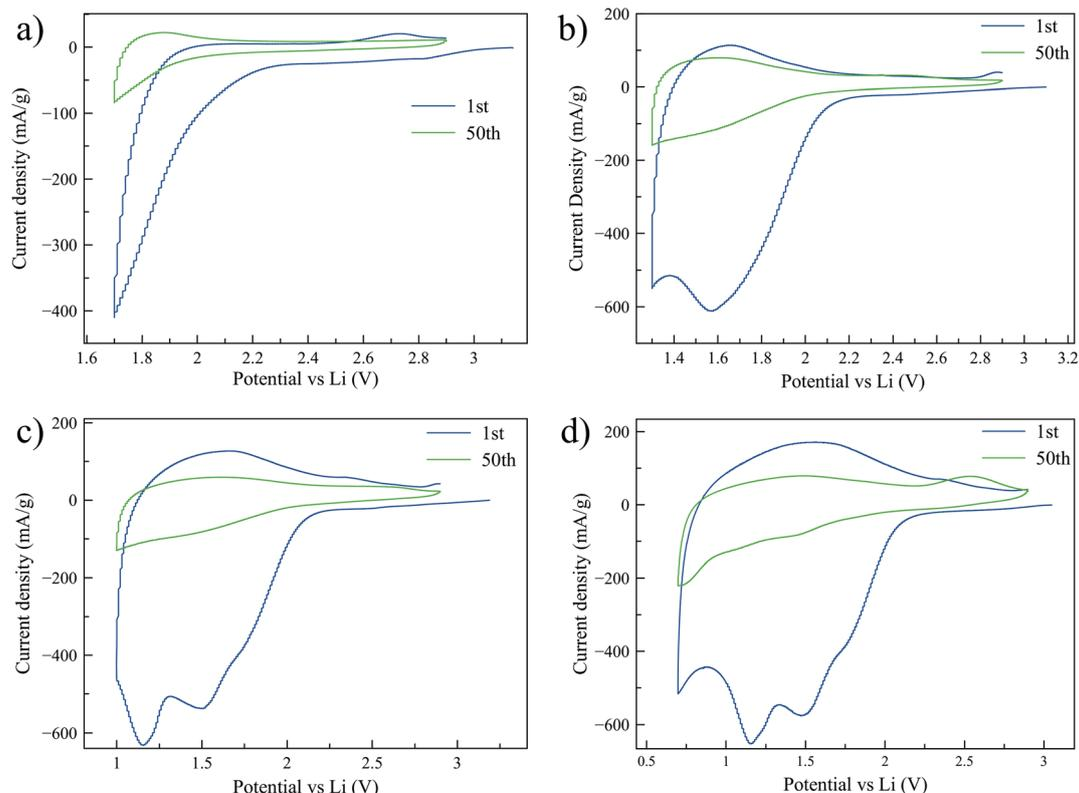
Fig. 4 Cyclic voltammograms performed with a three-electrode setup at  $0.3 \text{ mV s}^{-1}$  between 2.9 V and 1.7 V (a), 2.9 and 1.3 V (b), 2.9 and 1.0 V (c), and 2.9 and 0.7 V (d). The first and fiftieth cycle of each CV are shown in the graphs.
