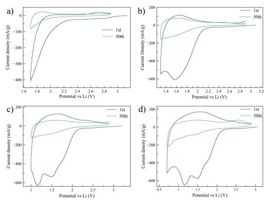
Fig. 4 Cyclic voltammetry scans performed with a three-electrode setup at  $0.3 \text{ mV} \text{ s}^{-1}$  between 2.9 V and 1.7 V (a), 2.9 and 1.3 V (b), 2.9 and 1.0 V (c), and 2.9 and 0.7 V (d). The first and fiftieth cycle of each CV are shown in the graphs.
