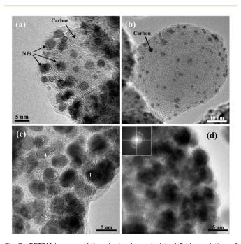
Fig. 7 BFTEM images of the electrode cycled to  $1.0~\rm V$  consisting of carbon particles incorporating smaller crystalline nanoparticles (a and b). HRTEM images used for d-spacing measurements (c). The inset shows the FFT diffractogram that corresponds to the whole image (d).
