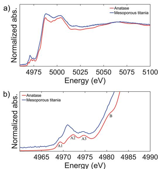
Fig. 2 XAS spectra of the anatase and the pristine mesoporous titania samples (a). The pre-edge features are highlighted (b). The absorption spectra are shifted in intensity for clarity.
