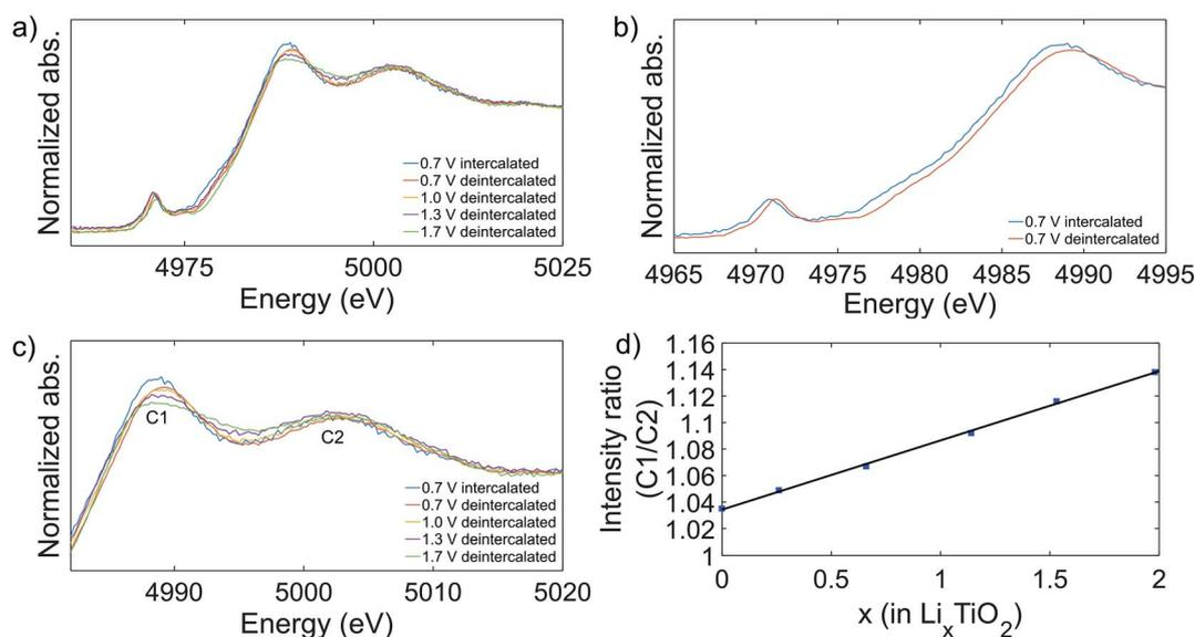
Fig. 5 XAS spectra of the cycled samples (a) and a comparison of the intercalated and the deintercalated state of the samples cycled to 0.7 V, showing a shift in the edge position (b). The post-edge region of the XAS spectra of pristine and cycled mesoporous titania is highlighted (c) and the effect of the lithium concentration on the peak intensity ratio C1/C2 (d). The point at  $x = 0$  is for the pristine sample.
