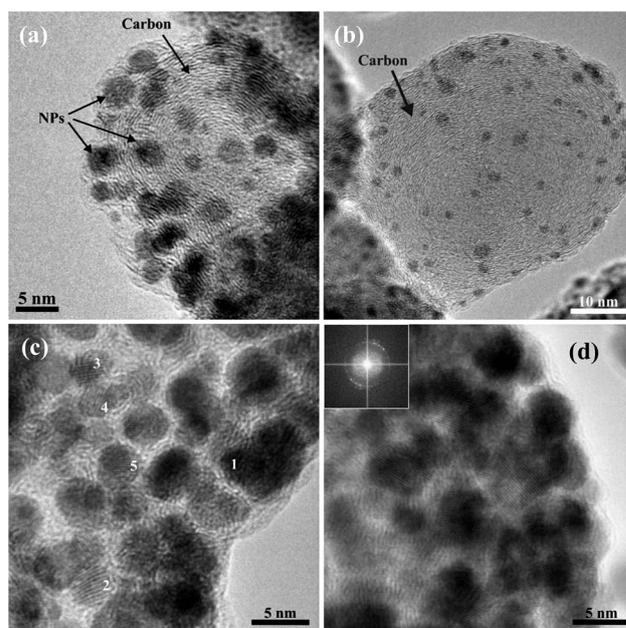
Fig. 7 BFTEM images of the electrode cycled to 1.0 V consisting of carbon particles incorporating smaller crystalline nanoparticles (a and b). HRTEM images used for  $d$ -spacing measurements (c). The inset shows the FFT diffractogram that corresponds to the whole image (d).
