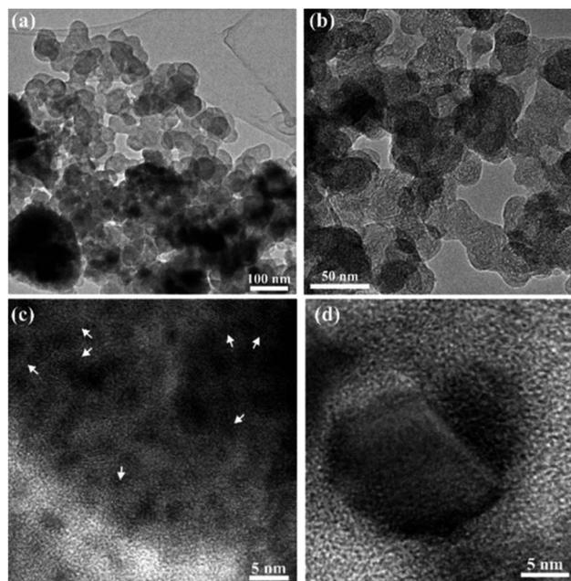
Fig. 6 Bright field TEM images of the electrode cycled to 1.7 V showing the overall morphology of the sample (a and b) and HR-TEM images showing the nanocrystalline anatase (c) and  $\text{LiTiO}_2$  (d).
