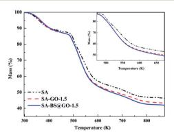
Fig. 6 TGA curves of the different membrane samples.
