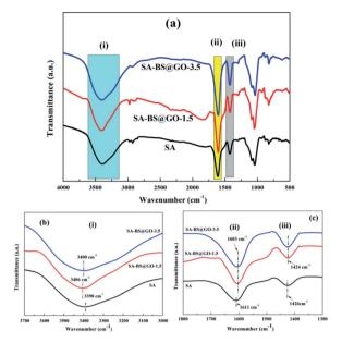
Fig. 4 FT-IR spectra of the SA and SA-BS@GO-X hybrid membranes: (a) whole spectra; (b) spectra of region (i); (c) spectra of regions (ii) and (iii).
