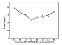
Fig. 10 Contact angles of the SA-BS@GO-X membranes with different mass ratios.
