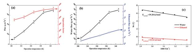
Fig. 12 Effects of operation temperature on the pervaporation performance of the SA-BS@GO-1.5 membrane: (a) total flux and separation factor; (b) water flux and ethanol flux; (c) Arrhenius plots for the permeation flux.
