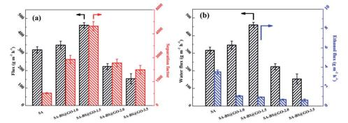
Fig. 11 Pervaporation results of the SA-BS@GO-X membranes: (a) total flux and separation factor; (b) water flux and ethanol flux.
