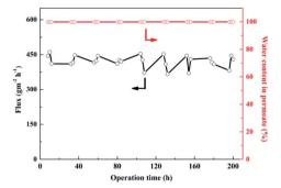
Fig. 15 Long-term operation evaluation of the SA-BS@GO-1.5 membrane
