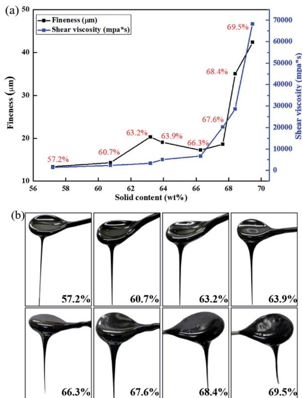
Fig. 2 (a) Fineness and viscosity of the cathode slurries as a function of solid content. (b) Flow diagram of slurries with different solid contents.
