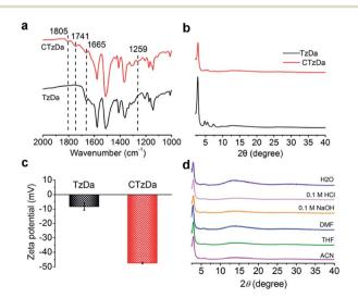
Fig. 2 (a) FTIR spectra of TaDa and CTzDa. (b) PXRD patterns of TaDa and CTzDa. (c) Zeta potential of TzDa and CTzDa. (d) PXRD patterns of CTzDa after immersing in various solvents.
