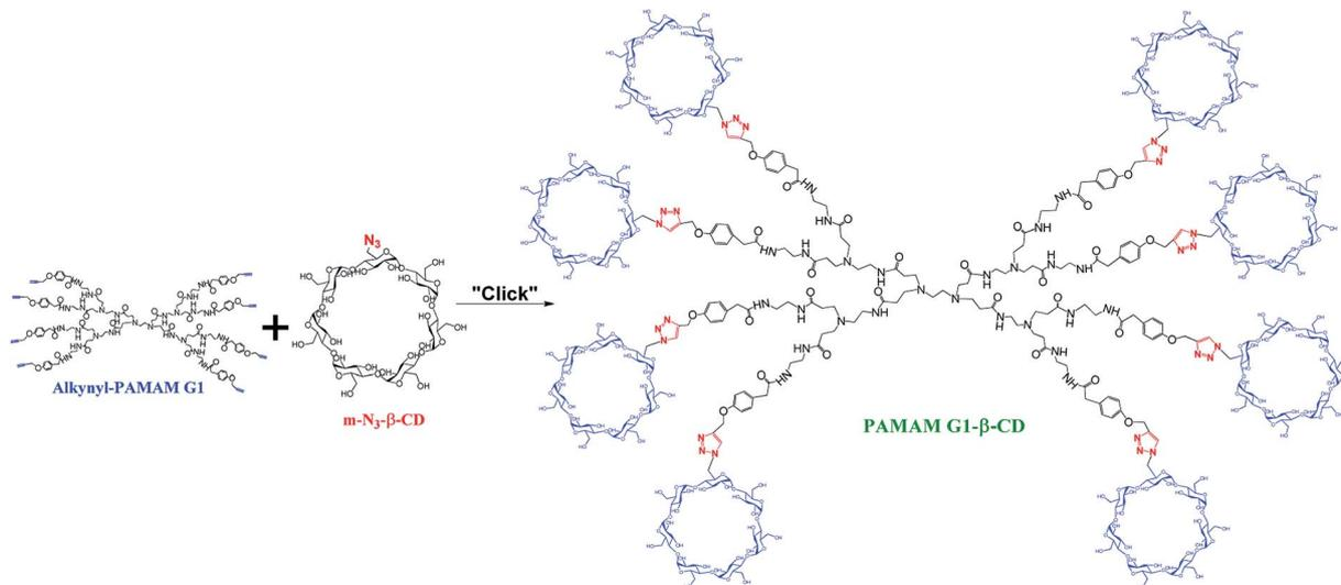
Scheme 3 Synthesis of PAMAM G1- $\beta$ -CD. Conditions: "Click"  $\text{CuSO}_4 \cdot 5\text{H}_2\text{O}$ ,  $\text{H}_2\text{Asc}$ , DMSO, 80 °C, 48 h.
