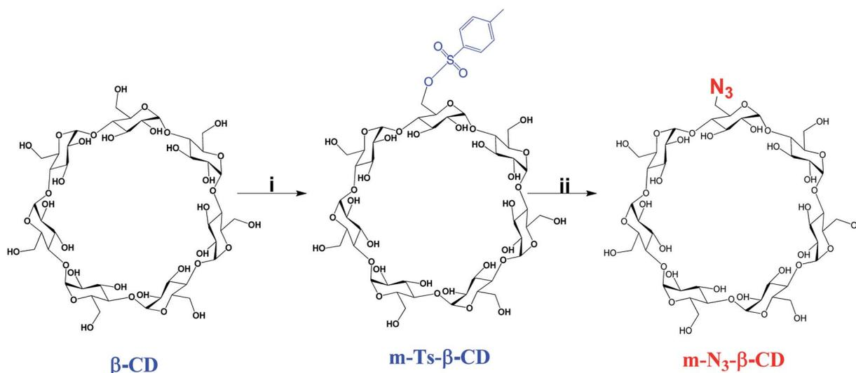
**Scheme 2** Synthesis of  $m-N_3$ - $\beta$ -CD. Conditions: (i)  $TsO_2/NaOH$ ,  $H_2O$ , 2 h, RT; (ii)  $NaN_3$ , DMF, 80 °C, 48 h.
