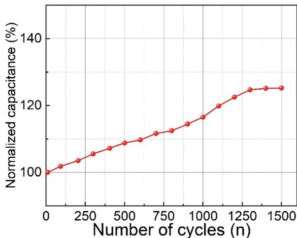
Fig. 8 Cyclic stability of CoFe<sub>2</sub>O<sub>4</sub> electrode prepared at RT at 0.5 mA cm<sup>-2</sup> current density.
