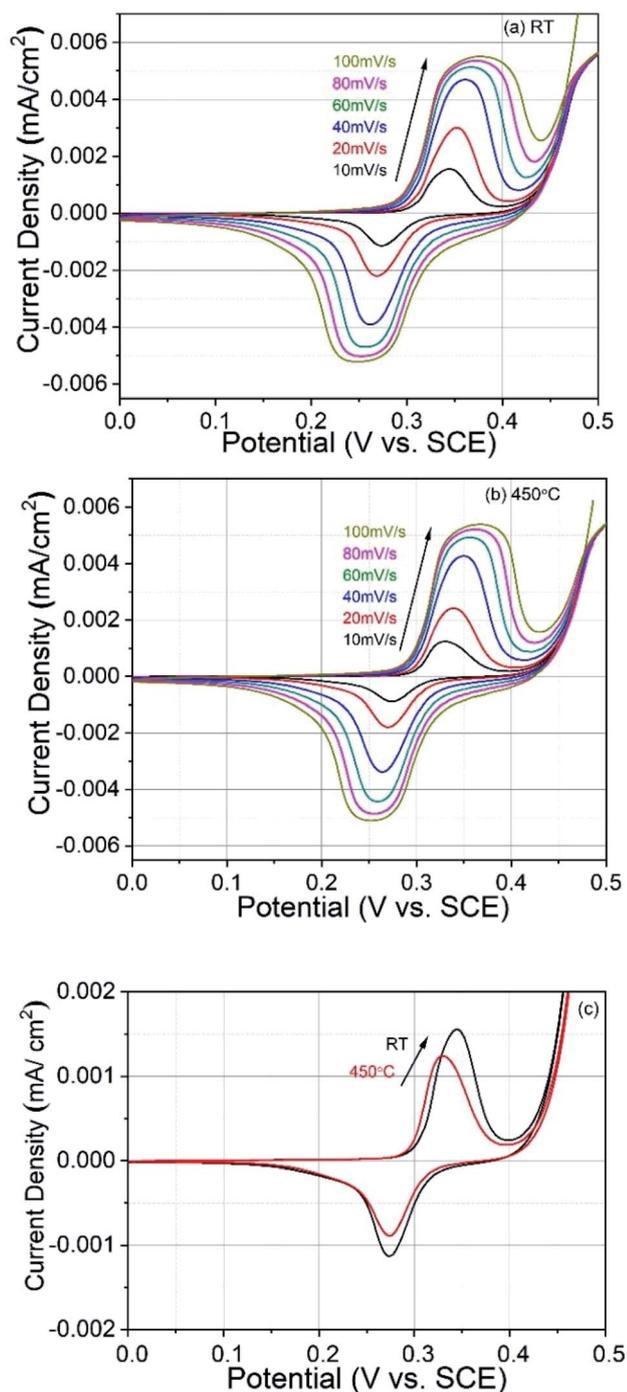
Fig. 5 Cyclic voltammograms at different scan rates of  $\text{CoFe}_2\text{O}_4$  electrodes prepared at (a) RT and (b) 450 °C. (c) CV plots of both electrodes at  $10 \text{ mV s}^{-1}$  scan rate for comparison.
