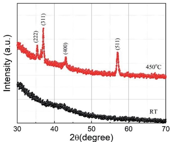
Fig. 2 X-ray diffraction patterns recorded for  $\text{CoFe}_2\text{O}_4$  thin films deposited at substrate temperatures of RT (black) and  $450^\circ\text{C}$  (red). The observed peaks in the scan are labelled with corresponding crystal planes of  $\text{CoFe}_2\text{O}_4$ .
