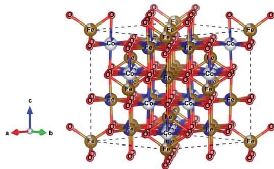
Fig. 1 Schematic crystal structure of spinel  $\text{CoFe}_2\text{O}_4$  ferrite ( $Fd\bar{3}m$  space group) showing Co and Fe cations as grey and gold spheres and O anions as red spheres, respectively.
