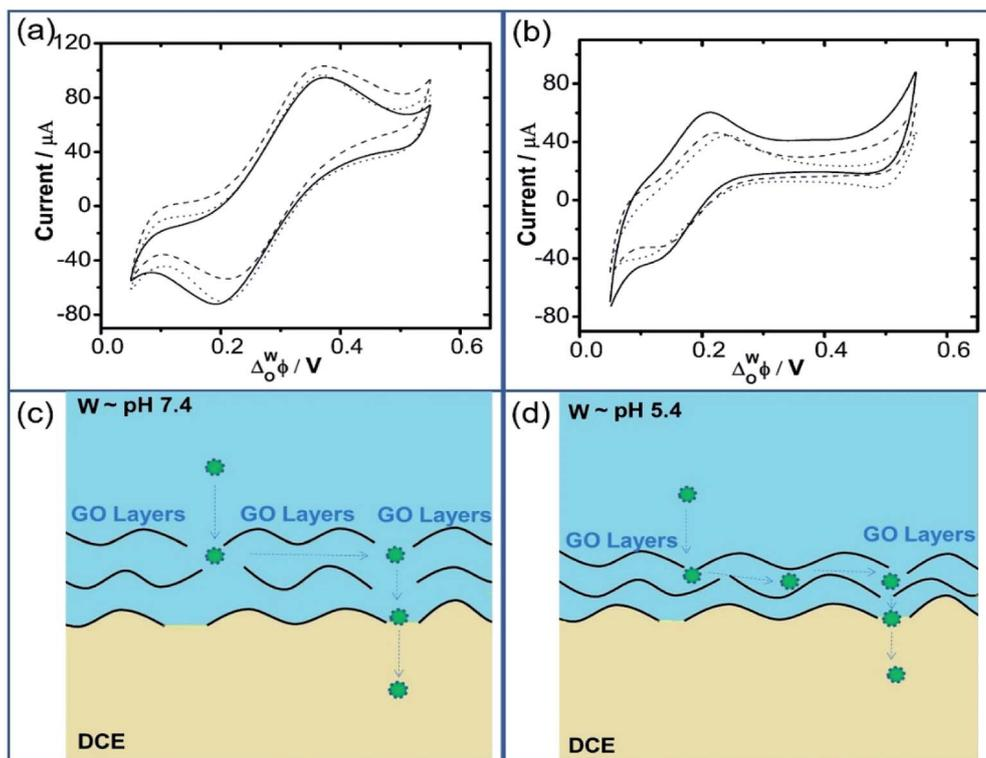
Fig. 5 Cyclic voltammograms for the transfer of 1 mM of (a)  $\text{TEA}^+$  and (b)  $\text{ClO}_4^-$  in the absence (solid line) and in the presence of GO ( $0.1 \text{ g L}^{-1}$ ) at pH  $\sim 5.4$  (dashed line) and  $\sim 7.4$  (dotted line); schemes for the ion transfer across the GO-layers-modified W/DCE interface under (c) pH  $\sim 5.4$  and (d) pH  $\sim 7.4$  by using cell 4.
