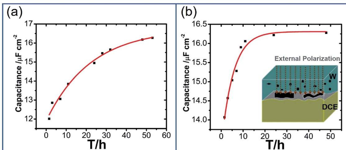
Fig. 4 The dependence between minimum capacitance ( $C_{\min}$ ) and time (a) without the external pre-polarization and (b) with the external pre-polarization at 0.2 V for 24 hours; the insets in (b) are the scheme for the adsorption of GO at the W/DCE interface with pre-polarization.
