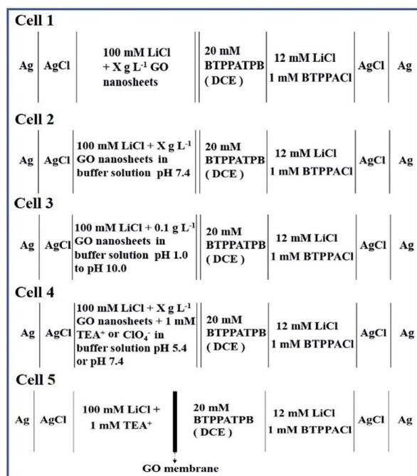
**Scheme 2** The electrochemical cells and their compositions used in the studies on the adsorption of GO (cells 1–3), as well as the ion transfer reactions occurring at the GO-layers-modified W/DCE interface (cell 4) and the GO-membrane-modified W/DCE interface (cell 5).
