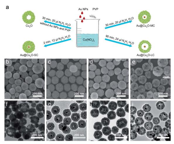
Fig. 1 (a) Schematic illustration of the synthetic process of different samples. (b–e) SEM, (f–i) TEM images of  $Cu_2O$ ,  $Au@Cu_2O$ -SC,  $Au@Cu_2O$ -MC,  $Au@Cu_2O$ -LC, respectively.
