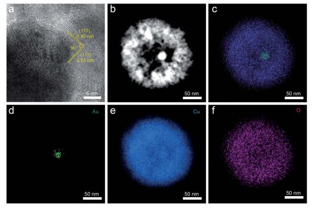
Fig. 2 (a) HRTEM, (b) DF-STEM and (c-f) EDS elemental mapping images of Au@Cu<sub>2</sub>O-MC.
