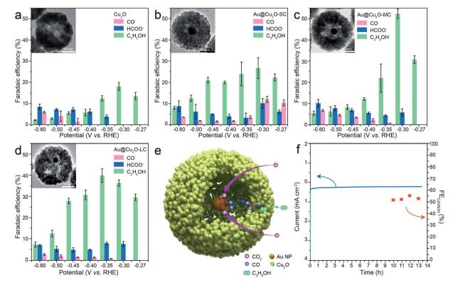
Fig. 4 (a–d) The faradaic efficiencies of carbon monoxide, formic acid, and ethanol from the  $CO_2RR$  products under a range of potentials of different samples. (e) Schematic illustration of tandem catalysis mechanism in the  $Au@Cu_2O$  cavity. (f) Time-dependent current density curve and  $FE_{C_3H_8OH}$  of  $Au@Cu_2O$ -MC in  $CO_2$ -saturated 0.1 M KHCO3 solution at -0.3 V vs. RHE.
