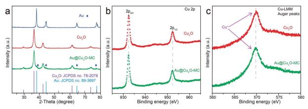
Fig. 3 (a) XRD patterns of different samples, (b) high-resolution Cu 2p and (c) Cu-LMM XPS spectra for Cu<sub>2</sub>O and Au@Cu<sub>2</sub>O-MC.
