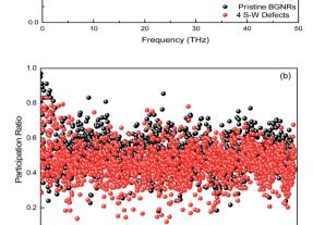
Fig. 6 The phonon participation ratio of BGNRs with different number of S-W defects at 300 K (a) AA-stacked; (b) AB-stacked.
