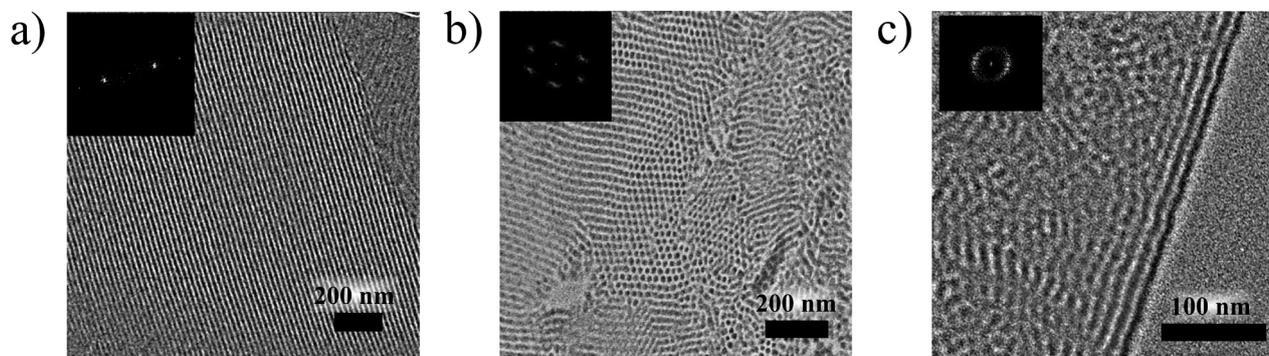
Fig. 4 The TEM images of cross-sections of the (a) pVP<sub>120</sub>-*b*-pPhM<sub>40</sub>, (b) pVP<sub>120</sub>-*b*-pPhM<sub>100</sub> and (c) pVP<sub>60</sub>-*b*-pPhM<sub>40</sub>-*b*-pVP<sub>60</sub> films. The samples were annealed at 140 °C for 3 h and then stained with iodine for 1 h.
