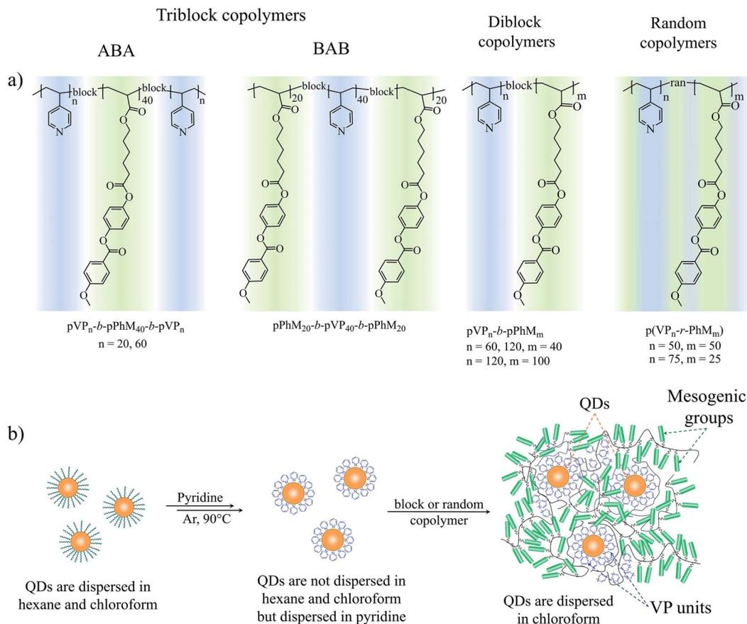
Fig. 1 (a) The chemical structure of the triblock, diblock and random copolymers. (b) The schematic route of the ligand exchange procedure.
