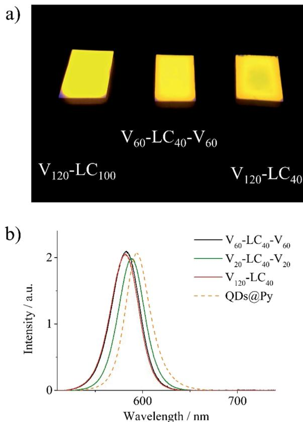
Fig. 8 (a) Photo of the composite films under UV irradiation ( $\lambda = 365$  nm,  $I = 1$  mW  $\text{cm}^{-2}$ ) and (b) fluorescence spectra of composites films and the pyridine solution of CdSe/ZnS QDs capped with pyridine (QDs@Py).
