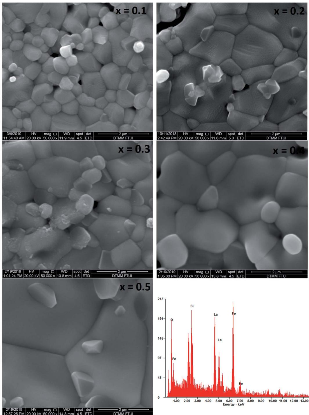
Fig. 4 SEM images of annealed  $\text{La}_{1-x}\text{Bi}_x\text{FeO}_3$  ceramics ( $x = 0.1, 0.2, 0.3, 0.4,$  and  $0.5$ ) and the energy dispersive X-ray spectrum of the  $\text{La}_{0.5}\text{Bi}_{0.5}\text{FeO}_3$  ceramic.
