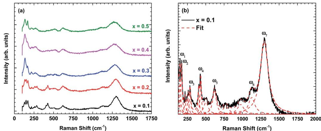
Fig. 3 (a) Raman scattering spectra of  $\text{La}_{1-x}\text{Bi}_x\text{FeO}_3$  ceramics ( $x = 0.1, 0.2, 0.3, 0.4,$  and  $0.5$ ) at room temperature and (b) the fitting results displayed for  $x = 0.1$  using standard Lorentzian profile.
