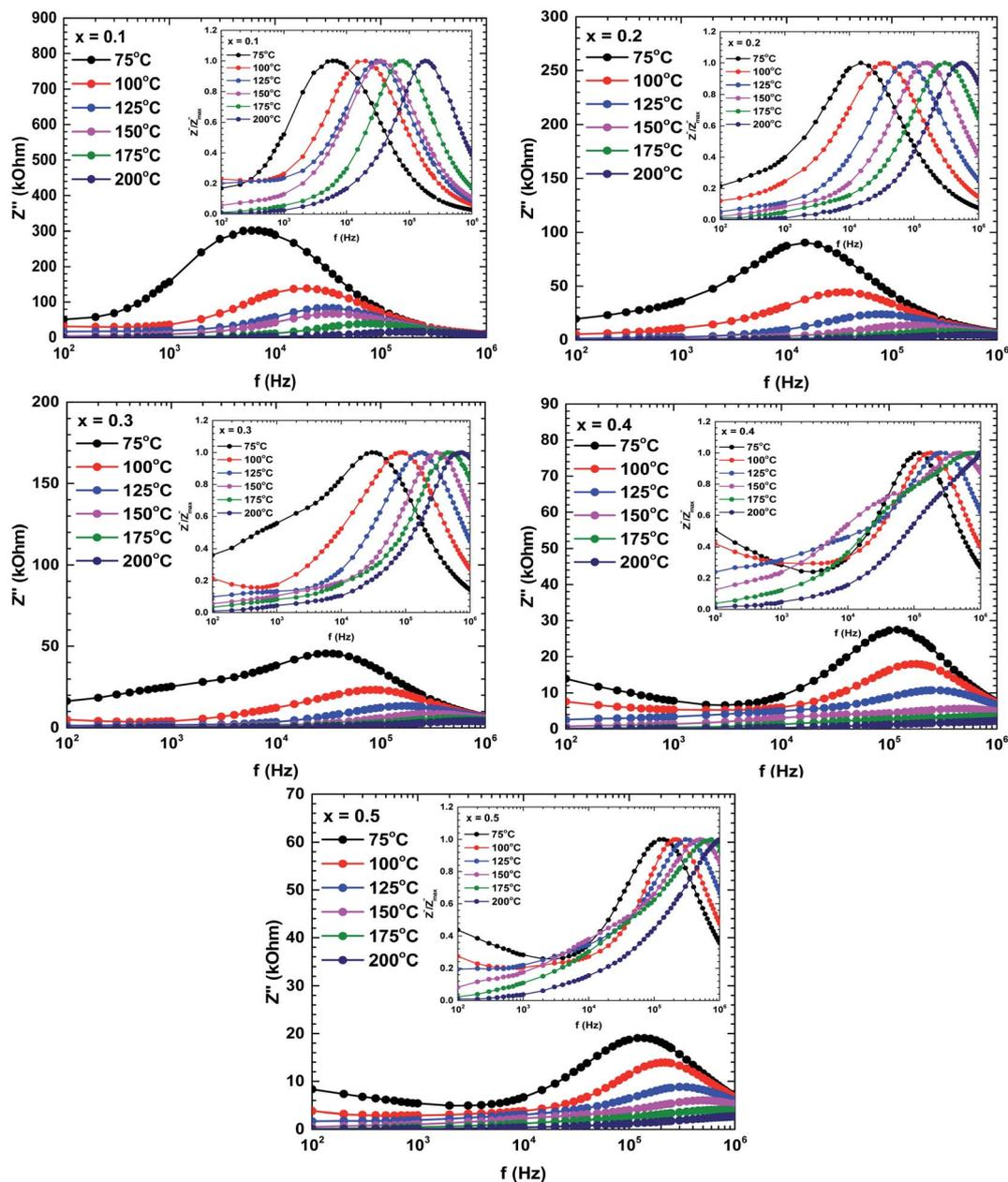
Fig. 7 Bode plots (imaginary impedances) of the  $\text{La}_{1-x}\text{Bi}_x\text{FeO}_3$  ceramics ( $x = 0.1, 0.2, 0.3, 0.4,$  and  $0.5$ ). The inset in each figure describes the normalized spectra of the imaginary impedance ( $Z''/Z''_{\text{max}}$ ) at different temperatures.
