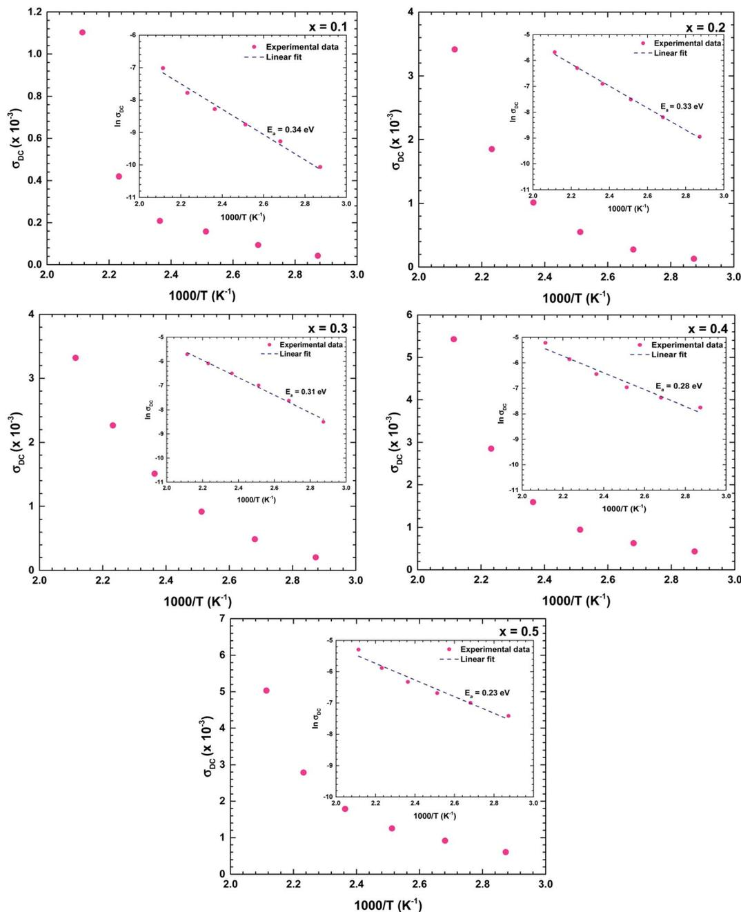
Fig. 11 Temperature dependence of the DC conductivity of the  $\text{La}_{1-x}\text{Bi}_x\text{FeO}_3$  ceramics ( $x = 0.1, 0.2, 0.3, 0.4,$  and  $0.5$ ). Insets describe the linear  $\ln(\sigma_{\text{DC}})$  vs.  $1/T$  plots, which satisfy the Arrhenius law.
