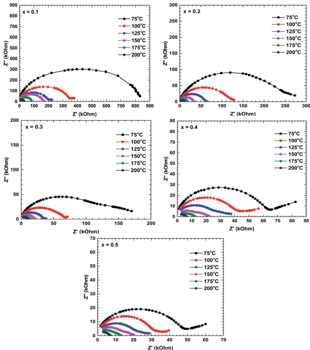
Fig. 5 Nyquist plots of the  $\text{La}_{1-x}\text{Bi}_x\text{FeO}_3$  ceramics ( $x = 0.1, 0.2, 0.3, 0.4,$  and  $0.5$ ).
