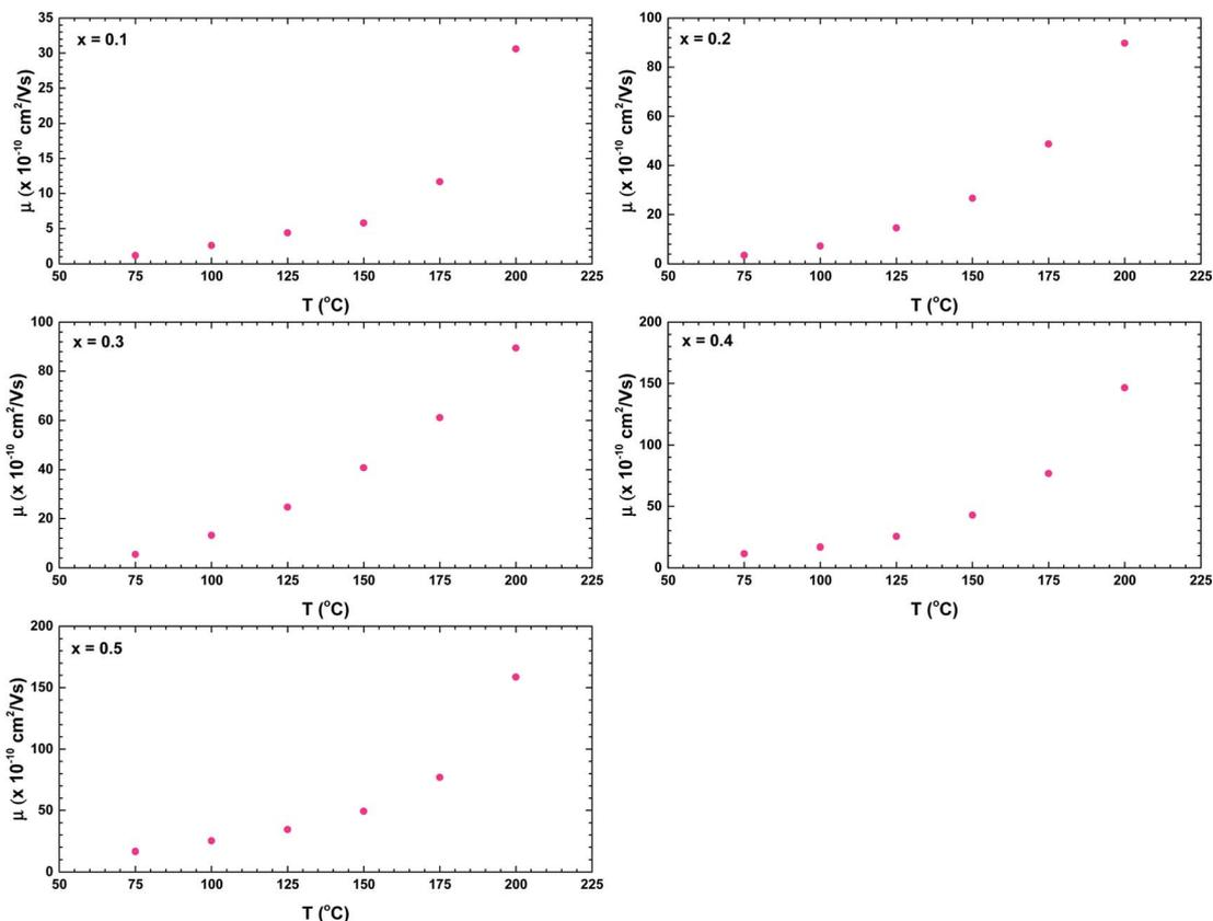
Fig. 12 Temperature dependences of the charge carriers mobilities of the  $\text{La}_{1-x}\text{Bi}_x\text{FeO}_3$  ceramics ( $x = 0.1, 0.2, 0.3, 0.4$ , and  $0.5$ ).
