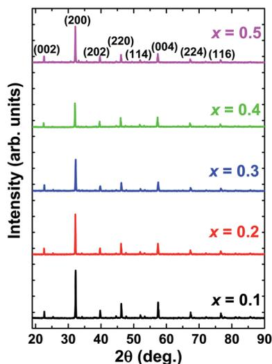
Fig. 1 XRD patterns of  $\text{La}_{1-x}\text{Bi}_x\text{FeO}_3$  ceramics ( $x = 0.1, 0.2, 0.3, 0.4,$  and  $0.5$ ).
