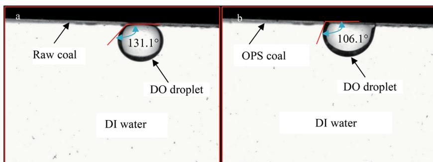
Fig. 13 Contact angle of coal–DO droplets in DI water: (a) raw coal and (b) OPS coal.
