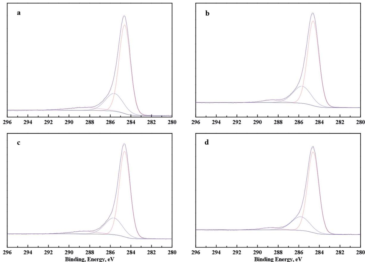
Fig. 10 XPS C 1s spectra of raw coal (a), DO coal (b), OPS coal (c), and OPS + DO coal (d).
