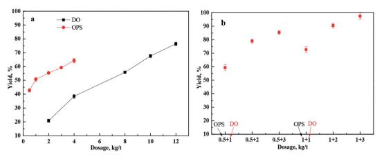
Fig. 2 Flotation results of coal samples as a function of DO (a), OPS (a), and OPS + DO (b) dose
