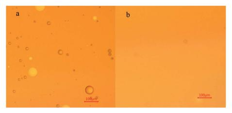
Fig. 5 Microscopic photograph of DO droplets in DI water (a) and OPS solution (b).
