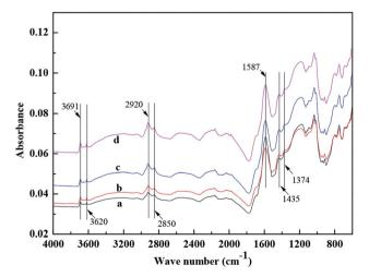
Fig. 8 ATR-FTIR of raw coal (a), DO coal (b), OPS coal (c), and OPS + DO coal (d).
