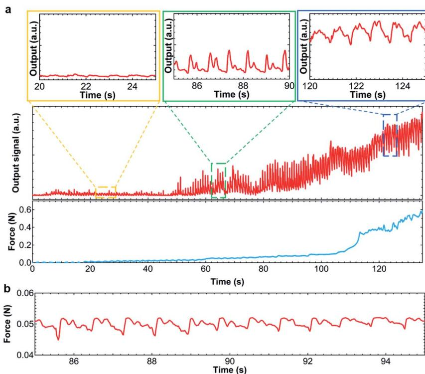
Fig. 5 (a) Heart pulse wave monitoring during one push deformation of the pump. Enlarged results for each time are also shown. Corresponding applied force to the output signal of the resistance change is also shown. (b) Real-time force to obtain the ideal heart pulse wave with two peaks. The increase of the output signal as a function of time is due to increase of the contact pressure of the sensor onto the wrist.
