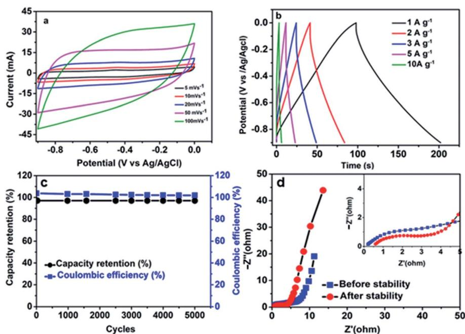
Fig. 6 (a) CV plots at scan rates of 5–100  $\text{mV s}^{-1}$ , (b) galvanostatic charge-discharge curves at different specific current, (c) cycling performance up to 5000 cycles and (d) EIS plots before after cycling test for ppAC electrode.
