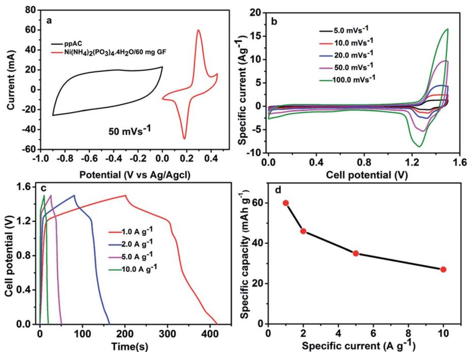
Fig. 7 (a) The CV curves of  $\text{Ni}(\text{NH}_4)_2(\text{PO}_3)_4 \cdot 4\text{H}_2\text{O}/60 \text{ mg GF}$  and ppAC at  $50 \text{ mV s}^{-1}$  scan rate in 3-electrode measurement, (b) CV curves at scan rates of  $5.0$ – $100.0 \text{ mV s}^{-1}$  for the device, (c) galvanostatic charge–discharge curves of asymmetric device at a specific current of  $1.0$ – $10.0 \text{ A g}^{-1}$ , and (d) specific capacity against specific current at  $1.0$ – $10.0 \text{ A g}^{-1}$  for the device.
