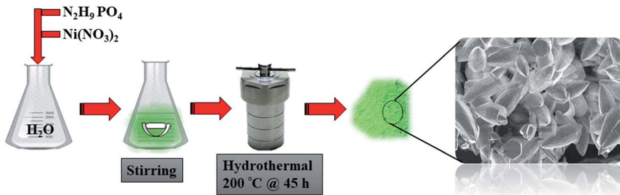
Scheme 1 Synthesis of \text{Ni}(\text{NH}_4)_2(\text{PO}_3)_4 \cdot 4\text{H}_2\text{O} and \text{Ni}(\text{NH}_4)_2(\text{PO}_3)_4 \cdot 4\text{H}_2\text{O}/\text{GF} composite.
