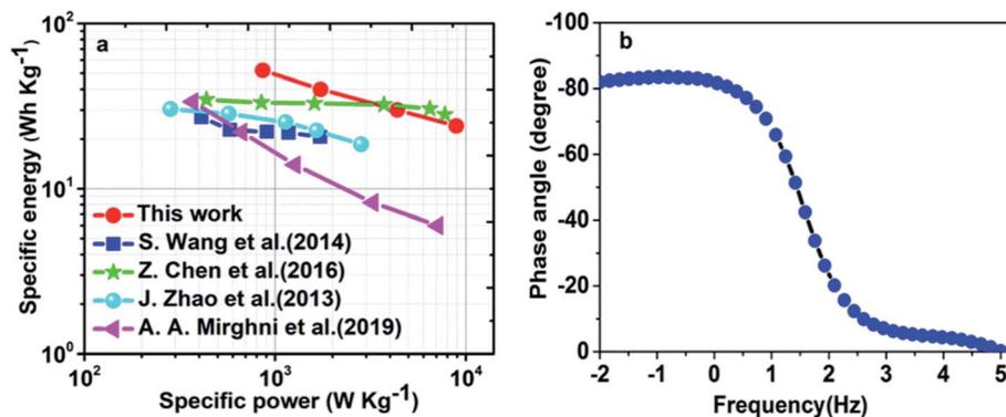
Fig. 9 (a) The Ragone plot of Ni(NH<sub>4</sub>)<sub>2</sub>(PO<sub>3</sub>)<sub>4</sub>·4H<sub>2</sub>O/60 mg GF/ppAC asymmetric cell and other similar works found in the literature and (b) the phase angle vs. frequency.
