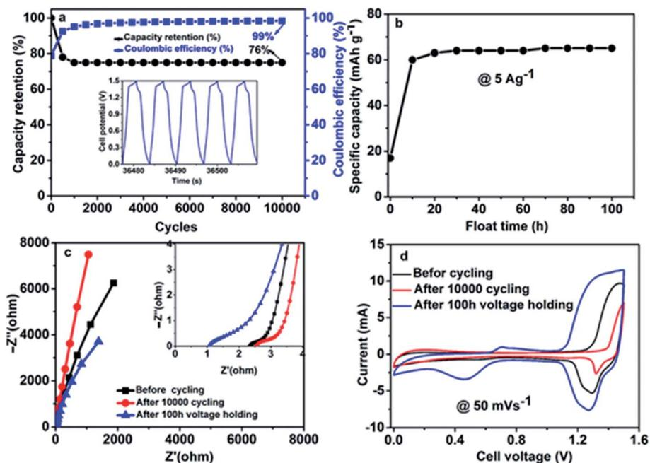
Fig. 8 (a) Capacity retention and coulombic efficiency measured with respect to cycle number at  $10 \text{ A g}^{-1}$ , (b) specific capacity vs. float time, (c) EIS comparison of  $\text{Ni}(\text{NH}_4)_2(\text{PO}_3)_4 \cdot 4\text{H}_2\text{O}/60 \text{ mg GF}/\text{ppAC}$  before cycling, after cycling and after the float time and, (d) CV comparison of  $\text{Ni}(\text{NH}_4)_2(\text{PO}_3)_4 \cdot 4\text{H}_2\text{O}/60$  before stability, after stability and after voltage holding.
