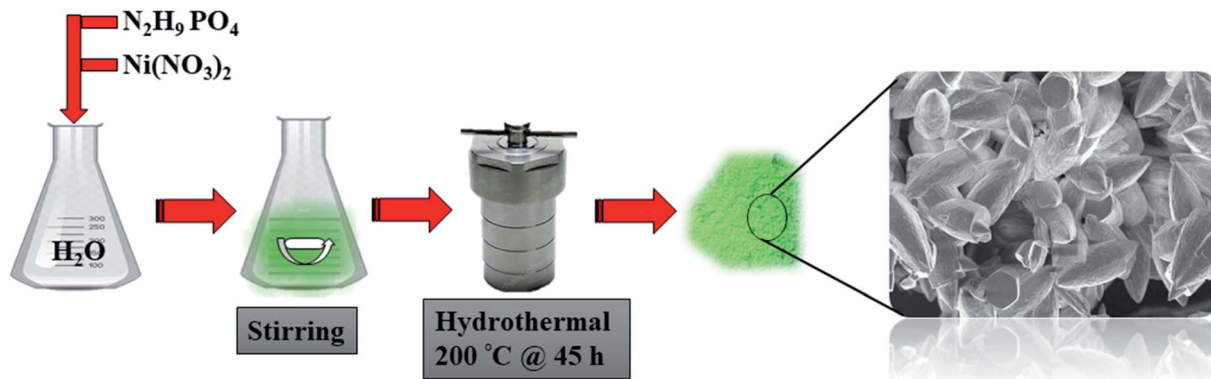
Scheme 1 Synthesis of \text{Ni}(\text{NH}_4)_2(\text{PO}_3)_4 \cdot 4\text{H}_2\text{O} and \text{Ni}(\text{NH}_4)_2(\text{PO}_3)_4 \cdot 4\text{H}_2\text{O} /GF composite.
