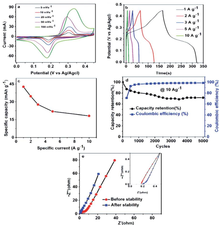
Fig. 5  $\text{Ni}(\text{NH}_4)_2(\text{PO}_3)_4 \cdot 4\text{H}_2\text{O}/60 \text{ mg GF}$  electrode (a) CV curve at scan rate of 5–100  $\text{mV s}^{-1}$ , (b) GCD plots at different specific currents, (c) specific capacity against specific current, (d) stability testing at 10.0  $\text{A g}^{-1}$  specific current and (e) EIS before and after stability.
