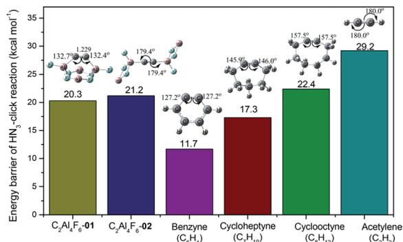
Fig. 3 Gibbs free energy barriers (in kcal mol<sup>-1</sup>) of the HN<sub>3</sub> click reaction with C<sub>2</sub>Al<sub>4</sub>F<sub>6</sub>-01, C<sub>2</sub>Al<sub>4</sub>F<sub>6</sub>-02, benzyne, cycloheptyne, cyclooctyne and acetylene at the CBS-QB3 level.
