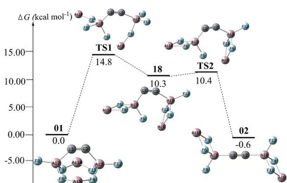
Fig. 4 The conversion pathways between C<sub>2</sub>Al<sub>4</sub>F<sub>6</sub>-01 and C<sub>2</sub>Al<sub>4</sub>F<sub>6</sub>-02 with the Gibbs free energy barriers at the CBS-QB3 level.
