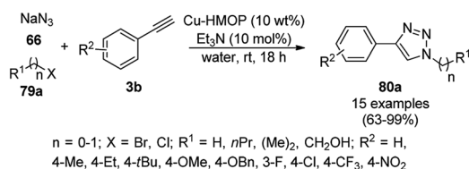
Scheme 29 Click reaction for the synthesis of triazoles (80a) catalyzed by Cu-HMOP.
