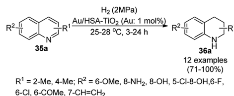
Scheme 13 Chemoselective hydrogenation of quinolines ( 35a ) catalyzed by Au NPs.
