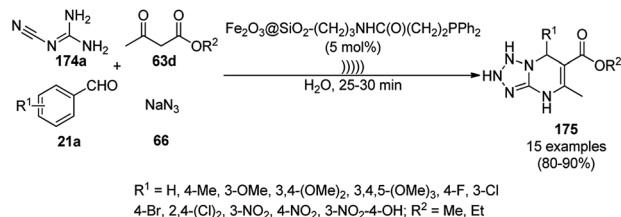
Scheme 90 Synthesis of tetrazolopyrimidines (175).
