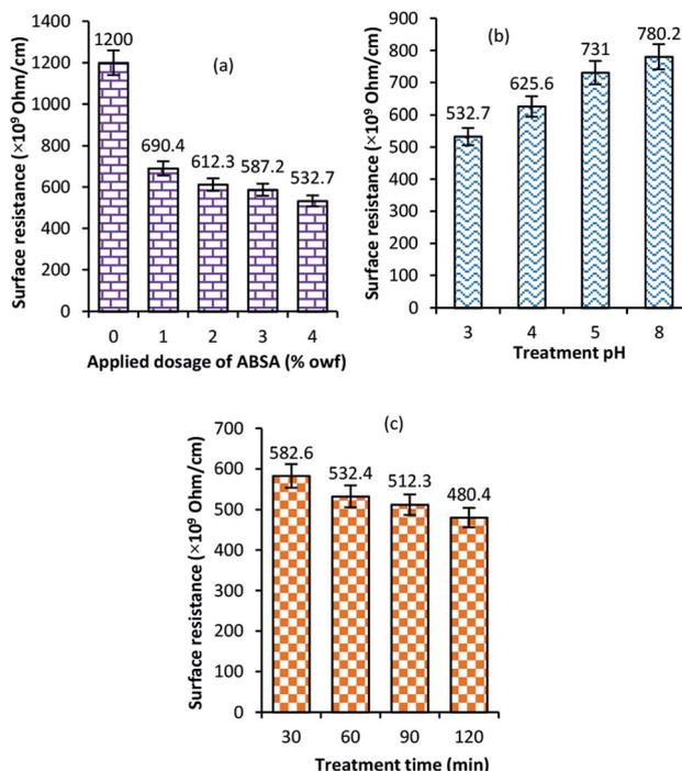
Fig. 1 Effect of applied dosage of ABSA (a), treatment pH (b) and time (c) on the average surface resistance of wool fabrics treated with ABSA.
