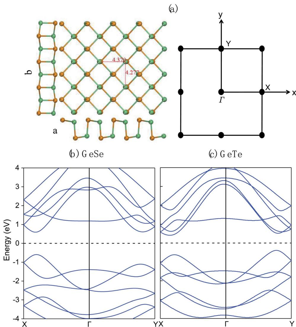
Fig. 1 (a) Top and side views of ML GeTe. (b and c) Band structure of the ML GeSe and GeTe. Green ball: Ge atom; brown ball: Te atom.  $\Gamma$ -Y and  $\Gamma$ -X represent the zigzag and armchair directions, respectively.
