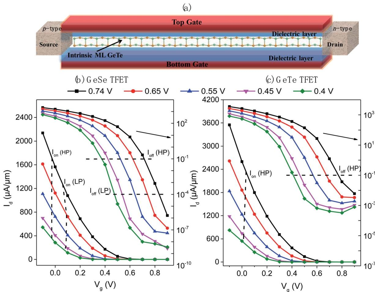
Fig. 2 (a) Device model of the ML GeTe TFET. Transfer characteristics of the ML GeSe (b) and GeTe (c) TFETs with  $L_g = 10$  nm at  $V_{dd}$  of 0.4–0.74 V. The ITRS requirements for HP and LP devices (2015 version) are given for comparison.  $N_S/N_D$  is  $0.1/5 \times 10^{13} \text{ cm}^{-2}$  for each TFETs.
