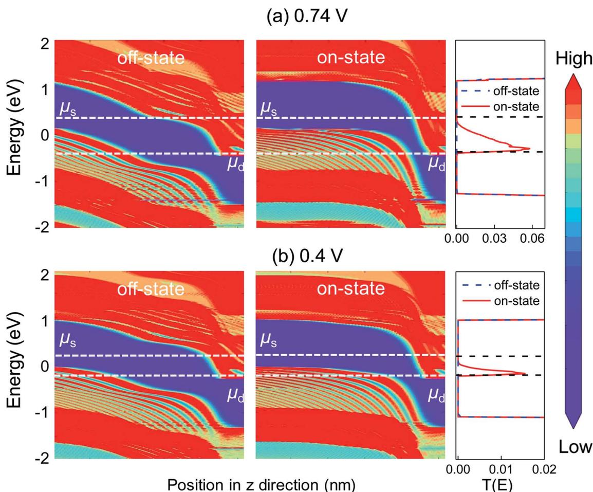
**Fig. 4** Local device density of states (LDDOS) and transport spectra of the ML GeTe TFET with a physical gate length of  $L_g = 10$  nm for HP application with  $N_s/N_D = 0.1/5 \times 10^{13}$  cm $^{-2}$  at the  $V_{dd}$  of 0.74 V (a) and 0.4 V (b).
