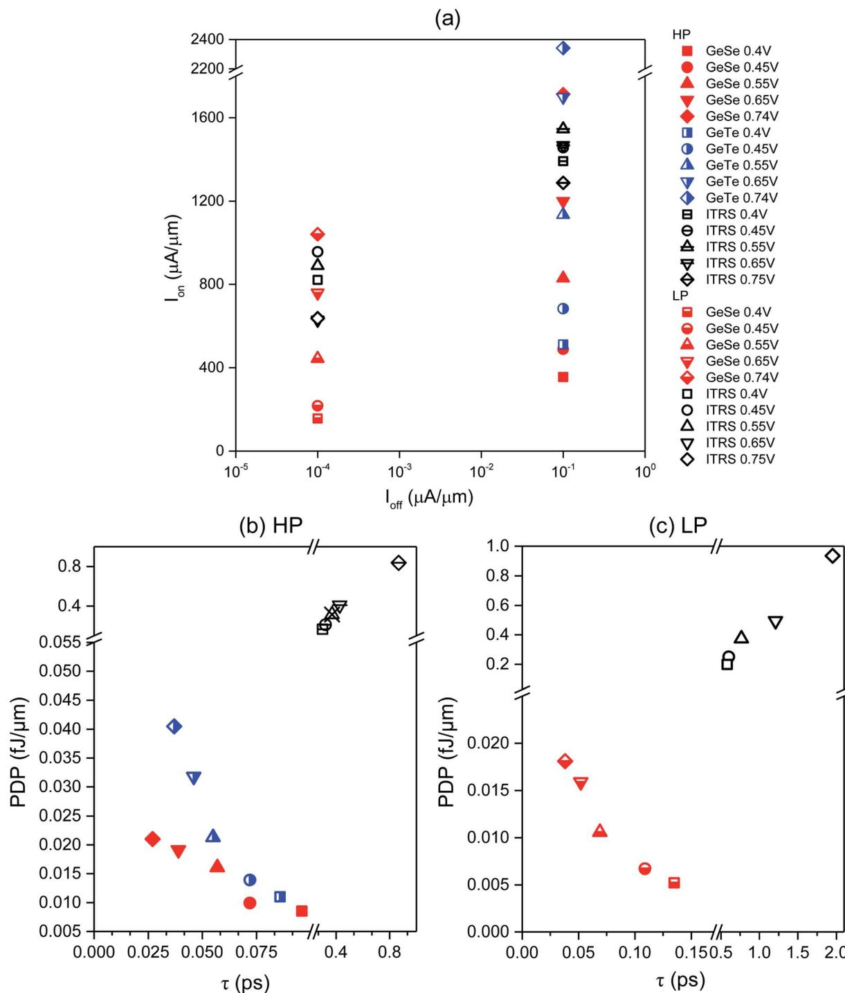
Fig. 3 (a)  $I_{on}$  vs.  $I_{off}$  and (b) and (c) delay time ( $\tau$ ) vs. power dissipation (PDP) of the ML GeSe and GeTe TFETs ( $V_{dd} = 0.4\text{--}0.74$  V) against those of the ITRS requirements for HP and LP devices (2015 version).
