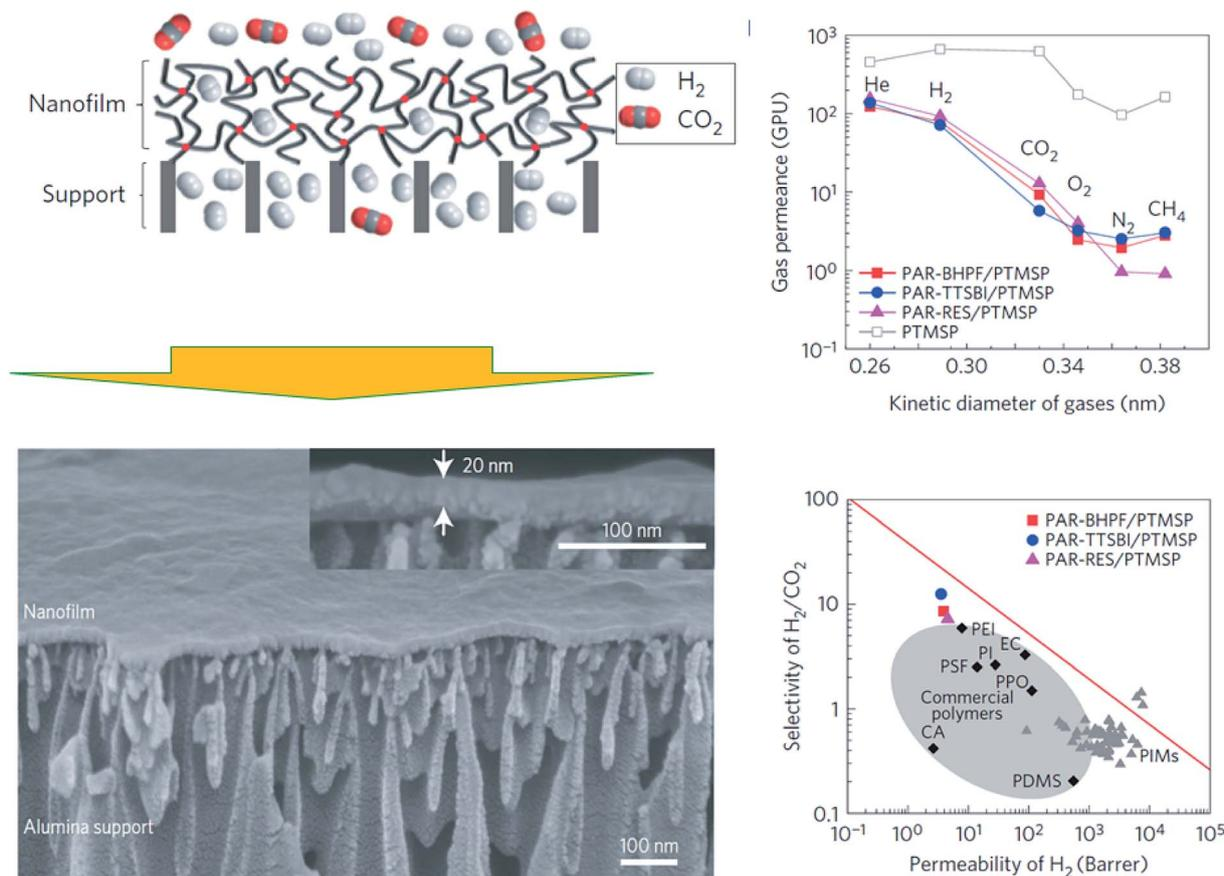
Fig. 8 Interfacial polymerization of polyacrylate-based nanofilms and their gas separation performance. Adapted from Jimenez-Solomon *et al.*<sup>99</sup>
