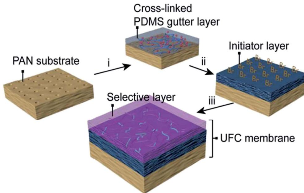
Fig. 4 Schematic depiction of the ultra-TFC membranes developed by Fu *et al.*<sup>51</sup>
