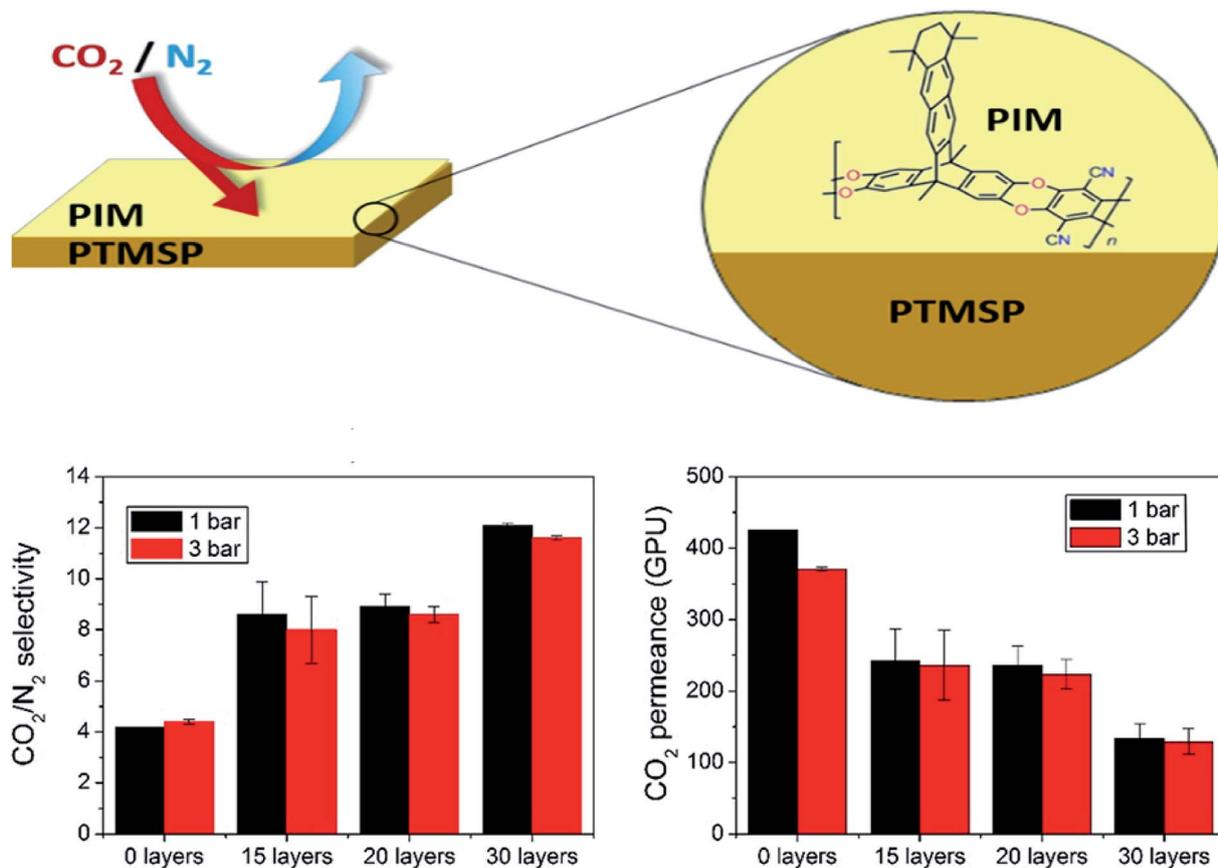
Fig. 9 Separation performance of ultrathin PIM-PTMSP membranes as a function of number of PIM layers. Adapted from Benito *et al.*<sup>110</sup>
