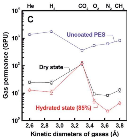
Fig. 7 Gas transport behavior of ultrathin GO membranes prepared by Kim *et al.*<sup>90</sup>
