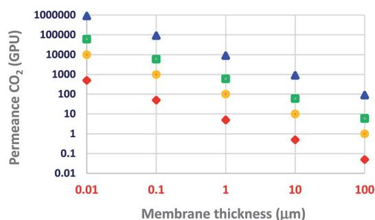
Fig. 3  $\text{CO}_2$  permeance as a function of membrane thickness: triangle, PIM-1; square, 6FDA-DAM; circle, Pebax® 1657; rhombus, polysulfone.<sup>29,41–43</sup>
