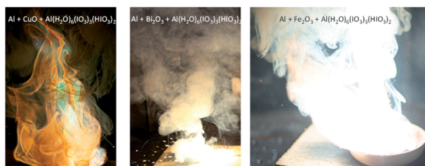
Fig. 4 Photographs of self-sustained reactions of aluminium fuel powder combined with the binary oxidizer combinations indicated. Note the copper oxide mixture produces green colour flames, bismuth oxide mixture shows particles ejected from the flame, and the iron oxide mixture produces bright white flames. Photographs were taken from a cell-phone camera.
