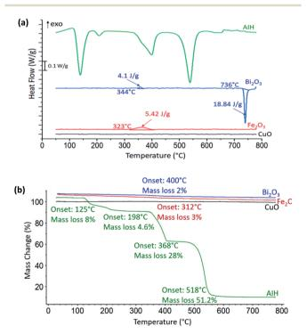
Fig. 2 (a) Heat flow as a function of temperature for CuO (black), Fe<sub>2</sub>O<sub>3</sub> (red), Bi<sub>2</sub>O<sub>3</sub> (blue), and AIH (green) at  $10^{\circ}$ C min<sup>-1</sup> heating rate in nitrogen environment. Note the scaling for heat flow is indicated on the graphic and onset temperature and enthalpy are also indicated. (b) Corresponding mass loss percentage curves with onset temperature and mass loss percentages indicated.
