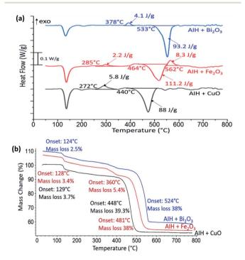
Fig. 3 (a) Heat flow as a function of temperature for AIH + CuO (black), AIH +  $Fe_2O_3$  (red) and AIH +  $Bi_2O_3$  (blue) in a nitrogen environment. Onset temperatures and enthalpies are indicated. (b) Corresponding mass loss percentage curves with onset temperatures and mass loss percentages indicated.
